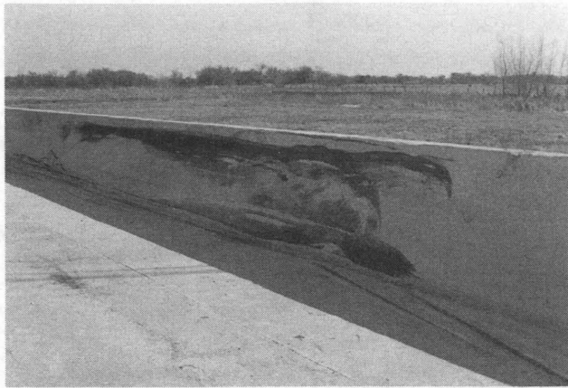
FIGURE 6 Damage to F-shape bridge railing and tractor trailer, Test 7069-10.
