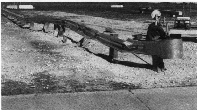
FIGURE 5 Damaged test vehicle and terminal after large car, redirection test.
