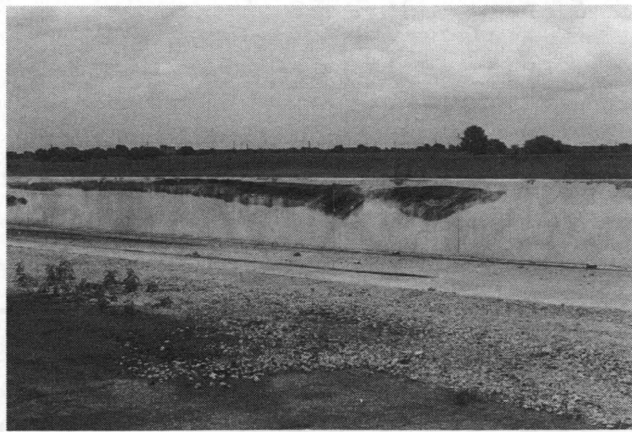
FIGURE 8 Damage to concrete parapet and tractor trailer, Test 7069-13.
