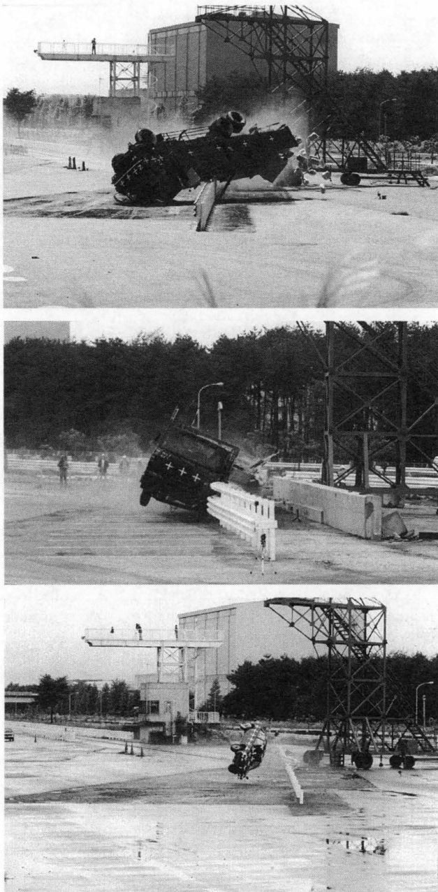
FIGURE 5 Results of impact test: (top) Gr-SS, (middle) Gr-SS Modified Type 2, (bottom) Gr-A'.
