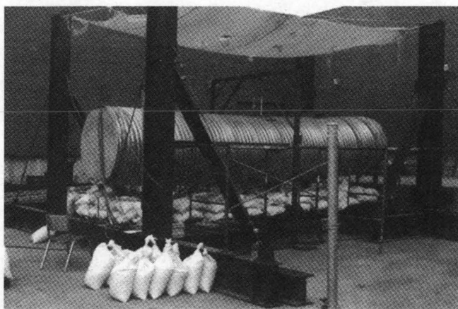
FIGURE 1 Load frame with ISU1 being tested.
