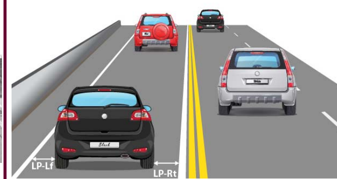
Figure 6. Lateral positioning of vehicle
