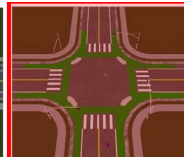
With islands and green pavement markings
