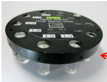
NASA water-film depth gauge
