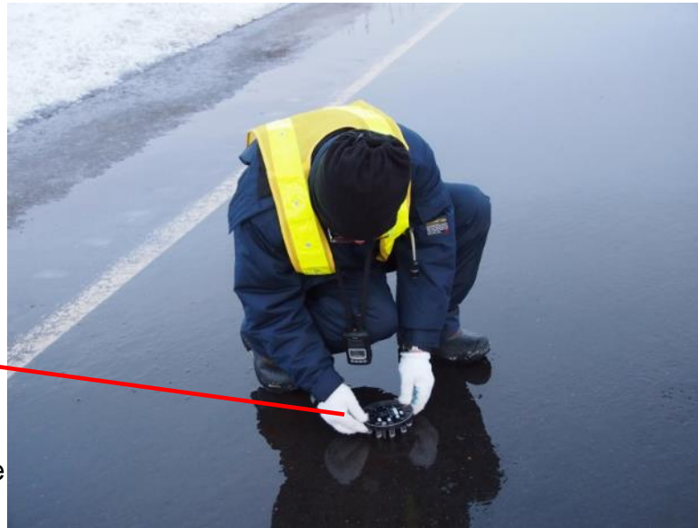
NASA water-film depth gauge
