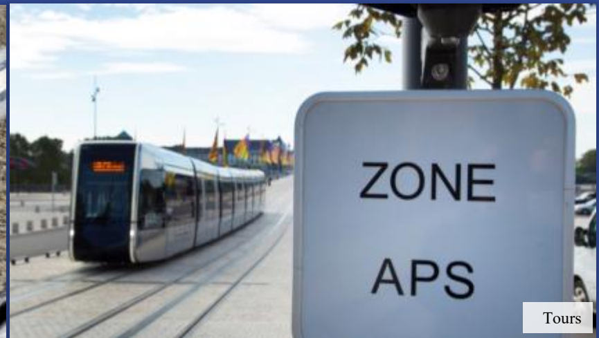
APS segmented street-level power rail
