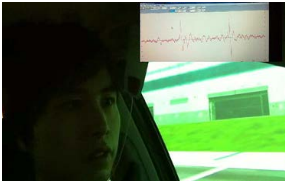
Figure 18 Example of detected eye blinking while the subject drove the driving simulator
