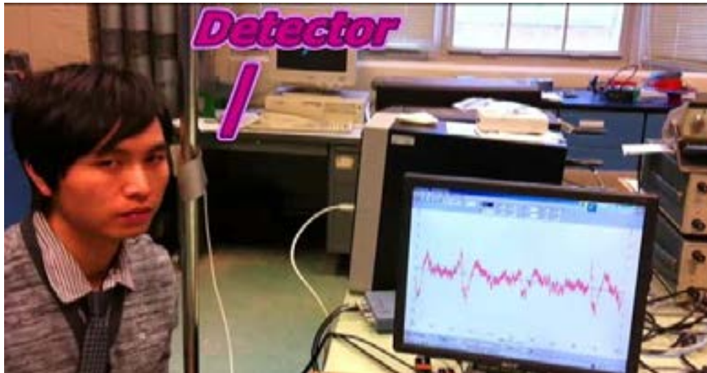
Figure 15 The detector is attached to a mounting pole for noncontact detection of eye blinking. Peaks in the displayed screen show the eye blinking activities.
