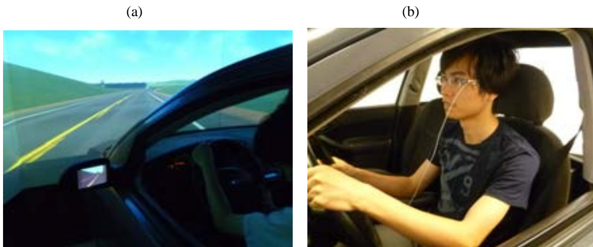
Figure 7 Driving fatigue detection: (a) High fidelity driving simulator; (b) photo of subject driving the driving simulator while being monitored by the eye blinking detection sensor.
