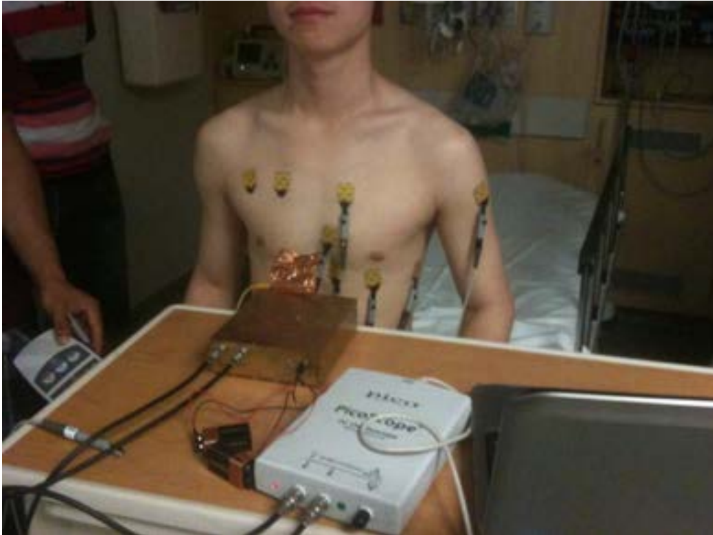
Figure 20 Comparison of non-contact ECG and clinic ECG
