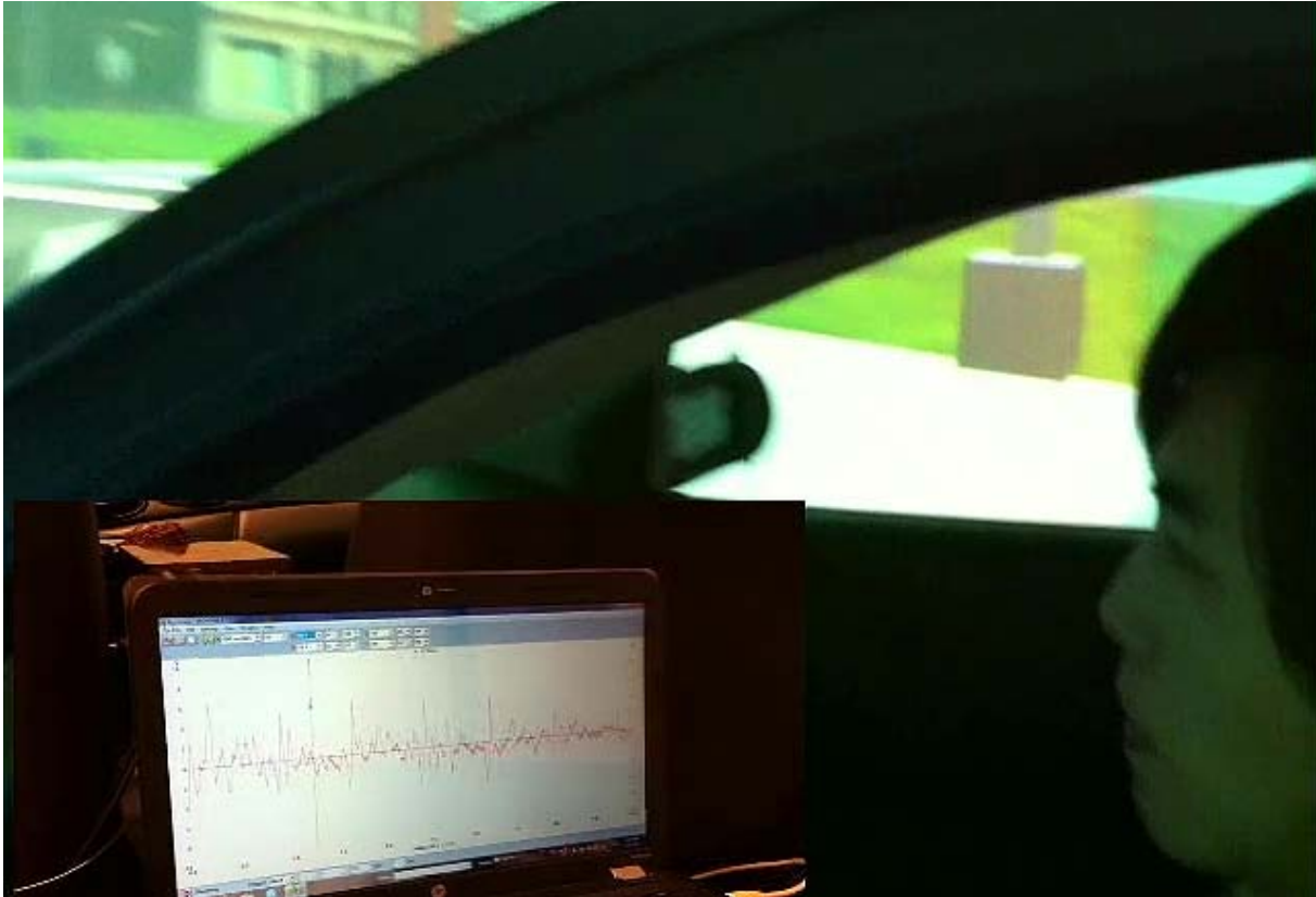
Figure 17 Measured ECG signal of subject while driving a driving simulator
