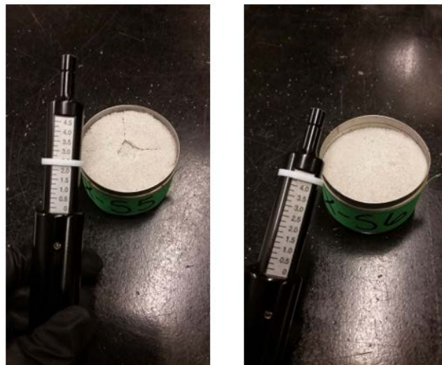
Figure 11. Penetrometer measurements of samples prepared for XRD analysis. On the left is clean sand treated with 0.5x BioCaN treatments and reads a strength of about 2.5 tsf (240 kPa). On the right is a clean sand treated with 2x BioCaN treatments and maxed out the instrument to produce a strength greater than 4.5 tsf (430 kPa). Note the soil crust is not broken in the sample cup on the right as the strength exceeded the capacity of the pocket penetrometer. Untreated clean sand produces 0 tsf (0 kPa) strength.
