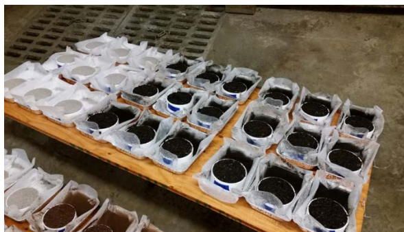
Figure 20. Sample cups after 30 minutes of rainfall were allowed to drain so that overtopping did not occur. During the experiment the samples were carefully monitored to make sure no overtopping was occurring.
