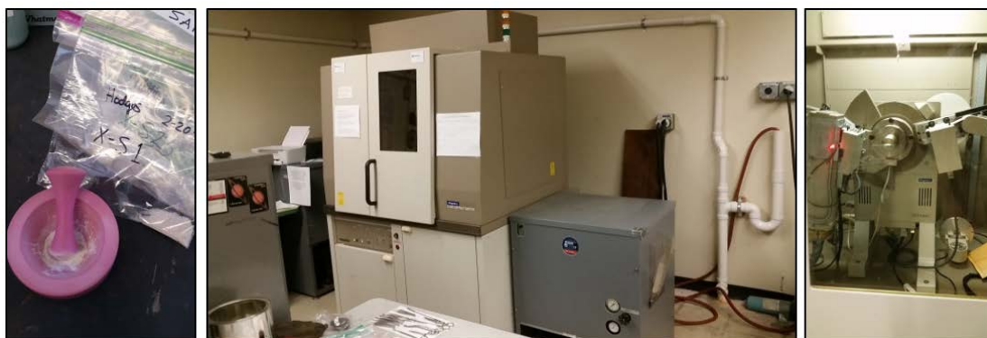
Figure 5. The X-Ray diffractometer used to identify crystalline structures in burned, unburned and sand untreated and treated soils for this study. The picture on the left is a pulverized sample ready for testing, the middle picture is the outside of the instrument and the picture on the right is the internal components while a scan is being run.
