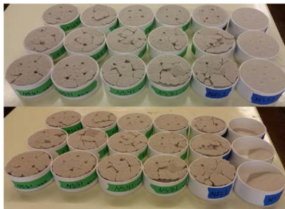
Figure 17. Sand specimen subjected to wind testing, the top image shows the samples prior to wind testing, the bottom image shows the samples after the wind erosion testing at 30 mph. The treatment type is shown on the labels and is the 3rd digit or the 1st number. Note that the control is on the right of the picture.
