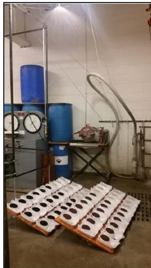
Figure 19. The image shows the rainfall simulator apparatus at the beginning of the BioCaN rainfall erosion test on 3 different soil types with 6 treatment levels conducted in triplicate.
