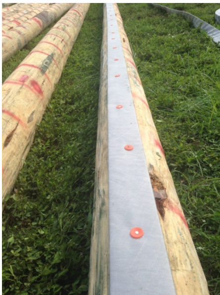
FIGURE 3.1 Drained timber pile prototype with one fastener per 0.3 m (12 in.).
