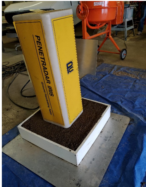
FIGURE (7) GPR Experiment to Measure Signal Attenuation
