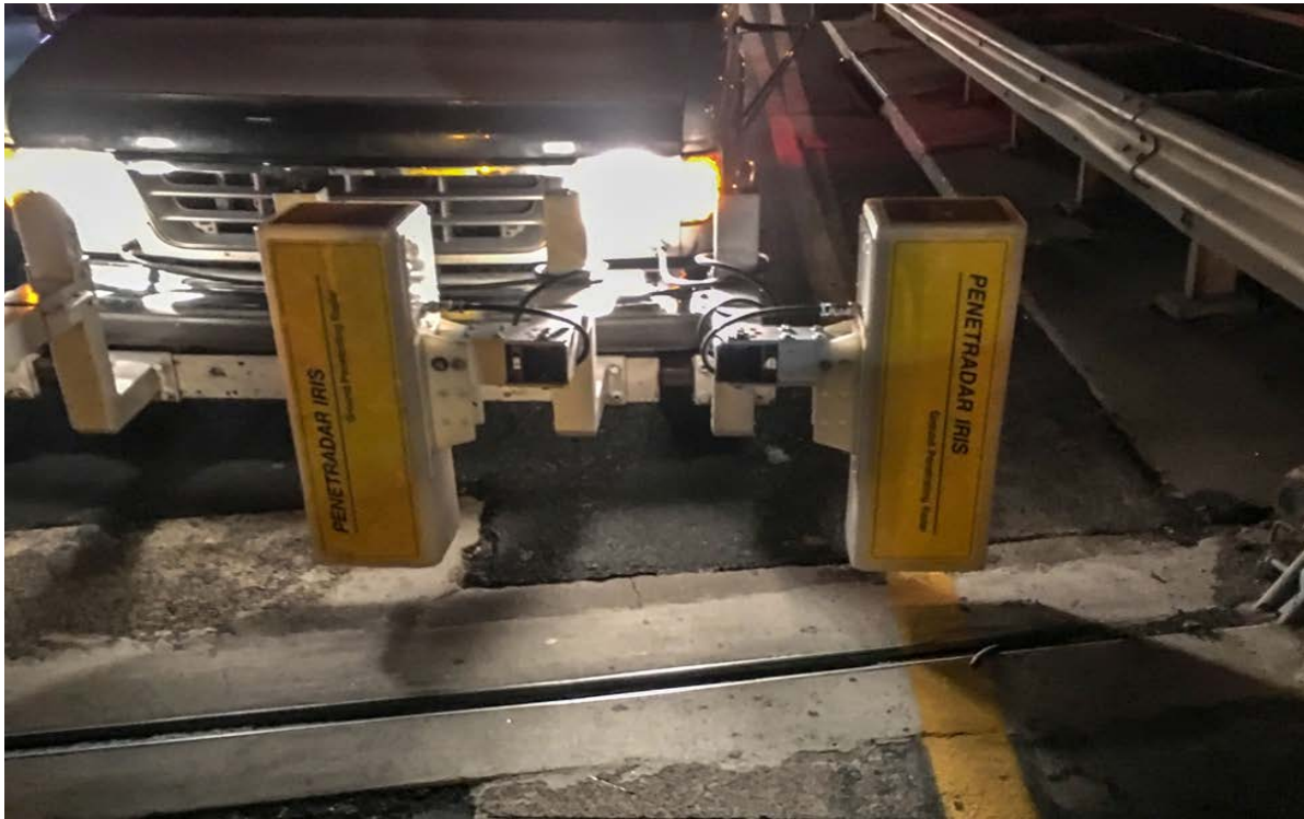
FIGURE (11) GPR Configuration used to Test the Sanger Avenue Bridge Deck
