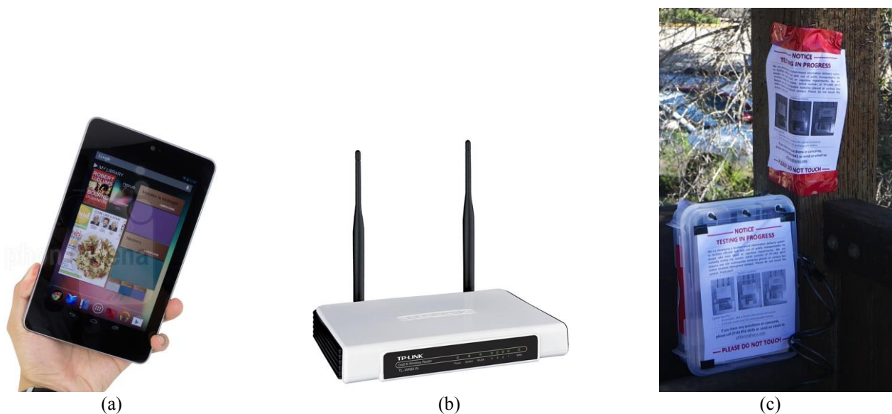
FIGURE 2 (a) The Nexus 7 tablet used as a client device. (b) The TP-LINK router functioning as access point (server). (c) TP-Link Access Point hosted in a plastic case and secured at a bus stop. Note the printed signs informing passers-by of the test in progress.
