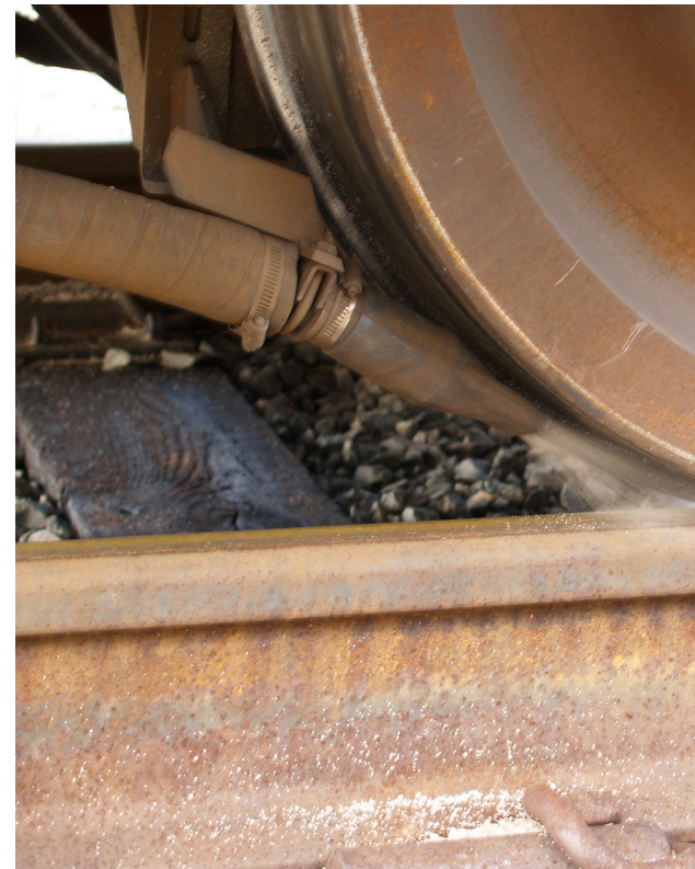
The technology deploys a variable amount of sand to allow the wheels to grip the rail.
