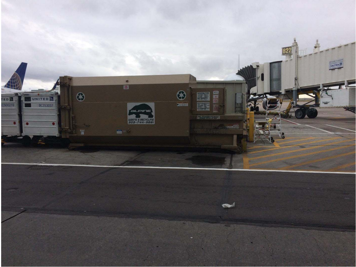
Figure 4: Ramp level recycling compactor, courtesy of Denver International Airport
