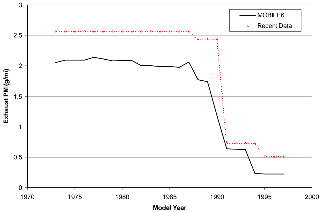
Comparison of MOBILE6 HDDV8B Exhaust PM Emissions to Results of Recent Test Programs
