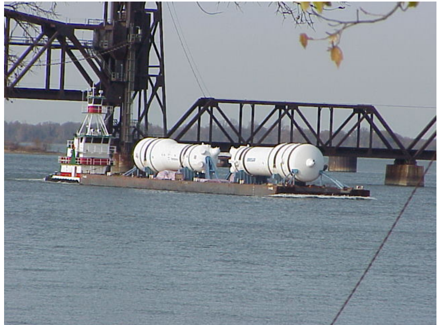
TVA steam generators en route to Sequoyah Nuclear plant on the Tennessee River.
