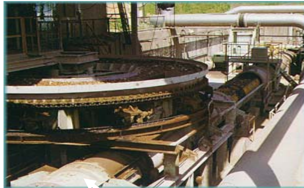
(b) Rotary loading of limestone at PCP inlet
