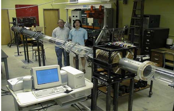
Figure 9. Test of PCP-LIM at the Power Electronic Laboratory of the University of Missouri-Columbia (From left to right, Professor Robert O'Connell and his former Ph.D student W. Plodpradista.)
