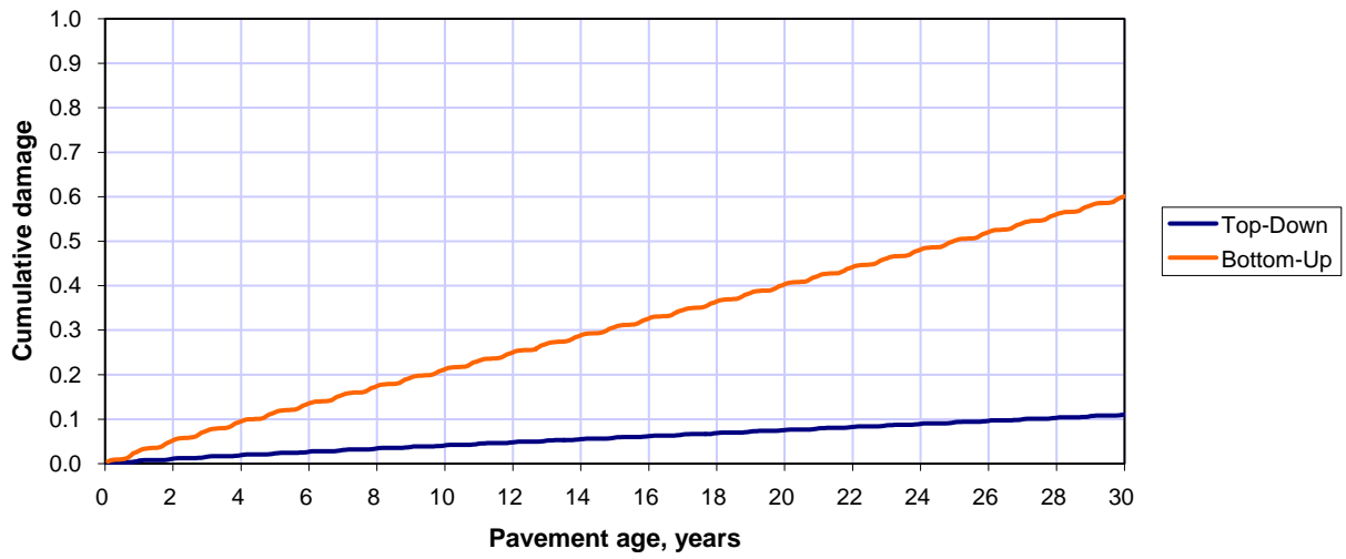
Figure 7. Plot of pavement age versus fatigue damage for unbonded JPCP overlay over existing PCC.
