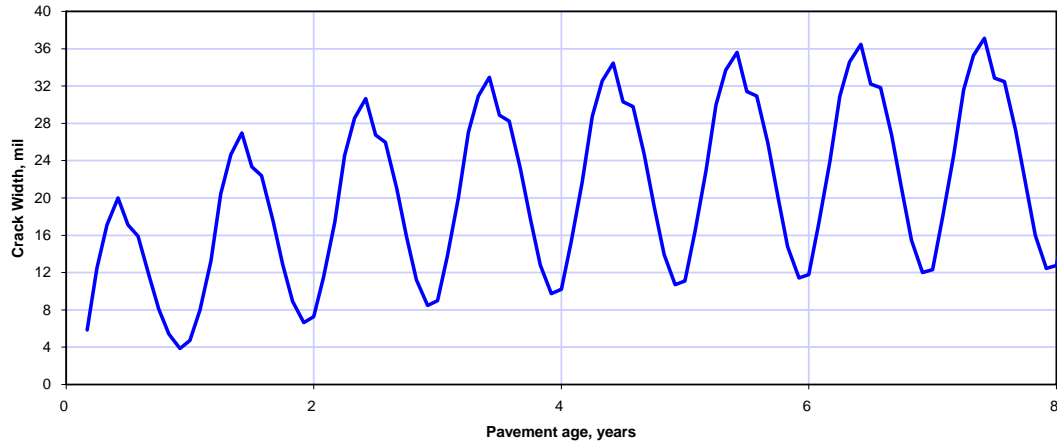
Figure 10. Plot of pavement age versus crack width for bonded PCC overlay over existing CRCP.
