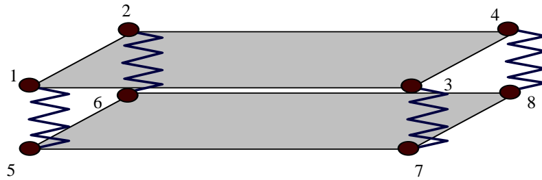
Figure 1.1. 8-noded finite element setup for Totsky Model.
