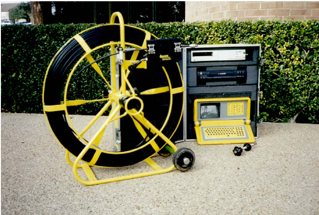
Figure 10. Camera system used for pipe inspections. SS-22
