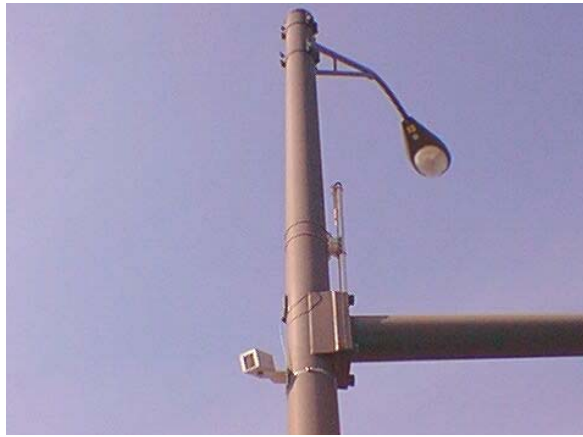
FIGURE 5 Doppler radar train detection system sensor.
