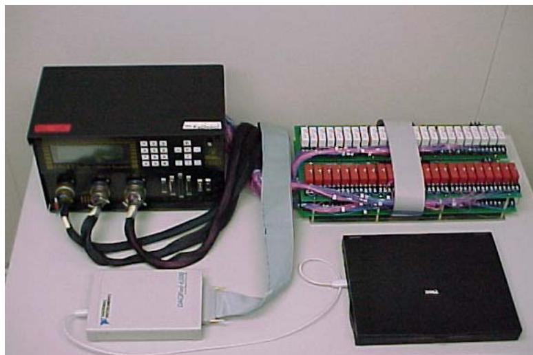
FIGURE 2 PC/Controller/CID simulation system.
