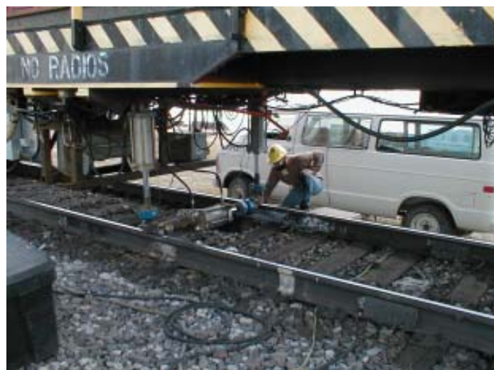
FIGURE 4-4 BiAST Installed in the Rail under TTCI's Track Loading Vehicle.
