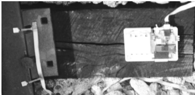
Figure 10. Controller box connected to two UAST's on a rail.
