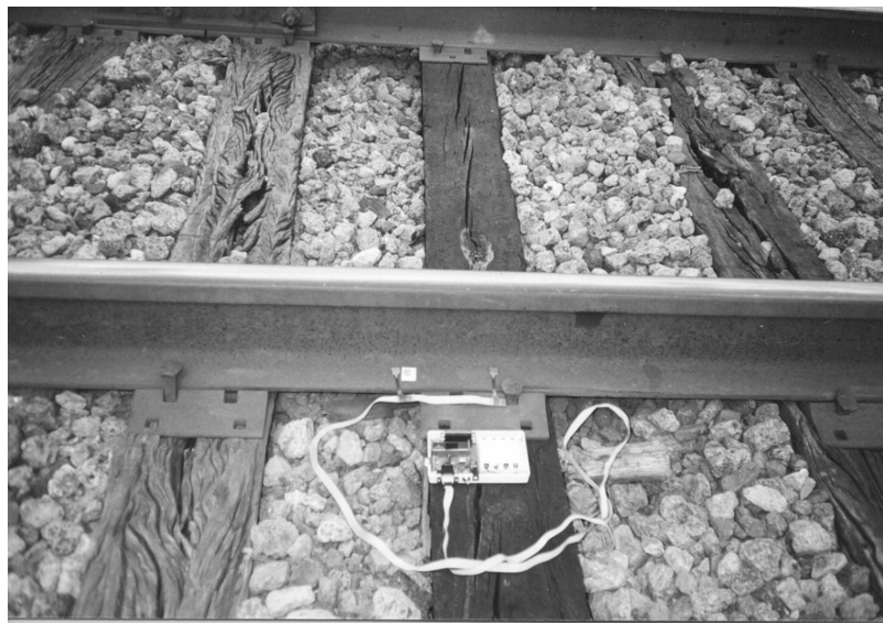
FIGURE ii. Strain data collection from a rail using UAST™ and a microcontroller.
