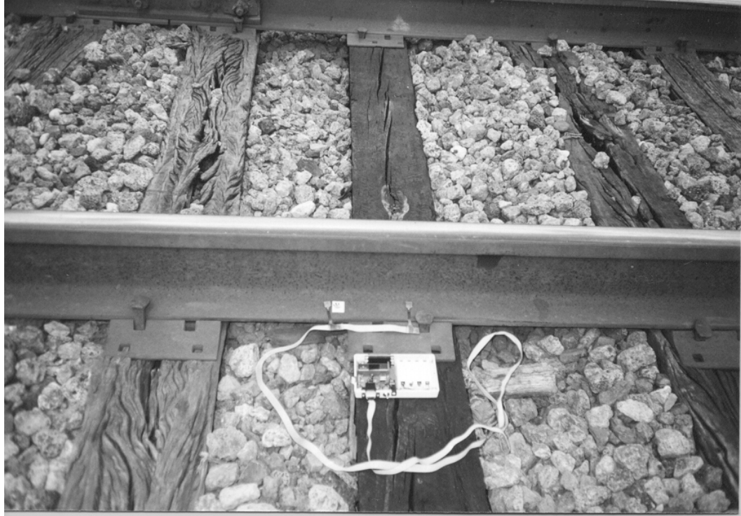
Figure 13. Strain data collection from a rail using UAST™ and a controller box.
