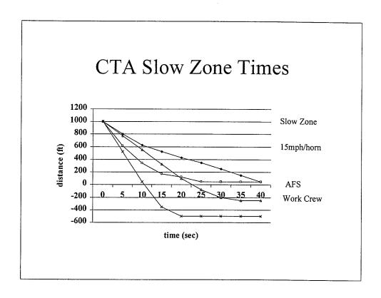
The graph illustrates the four scenarios discussed on the prior chart. The plot shows the position of the train relative to the flagman (AFS at 0ft) as a function of time referenced to 0 seconds (train at 1000ft from the flagman). Again, the work crew is on the tracks at -200ft relative to the flagman.
