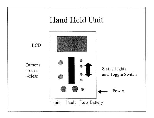
The HHU is designed to allow remote operation and communications while wearing gloves. A recessed power switch activates the unit. A low battery indicator and a fault light (together with the display panel) provide system status information.
