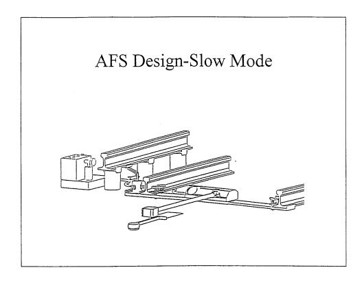
Upon the command from the foreman the AFMU sets to the Slow Mode. The pole with the red light and flag folds towards the train, and only the clear light is visible. At the same time the trip staff rotates away from the rail to not switch on the train brakes. If the mode has not been not reset once the train has passed and sufficient time has elapsed, then the AFMU will signal the foreman that it is about to automatically reset to the Stop Mode.
