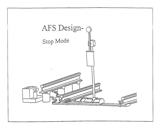
The Stop Mode is the default configuration of the AFMU. In the Stop Mode the trip staff is in position to automatically brake a train, if necessary. Also, the red light and flag are over the center of the track and oscillating. When a train is detected a long blast of the horn is emitted. In an emergency the oscillation is more rapid and continual short blasts of the horn are emitted. At the command of the foreman the AFMU sets to the Slow Mode.
