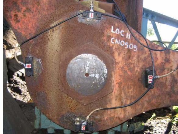
Active, or growing, flaws in safety critical structures emit acoustic emission (AE) under load while dormant flaws do not emit AE.
