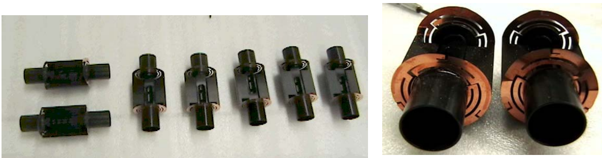
Figure 7. Fabricated Mechanical Parts for Prototype Accelerometer
