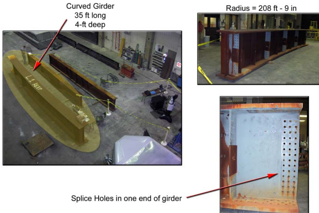
FIGURE 13 Curved girder specimen used for laboratory testing.
