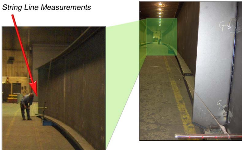
FIGURE 4 Conventional string line or other manual measurements can be eliminated.
