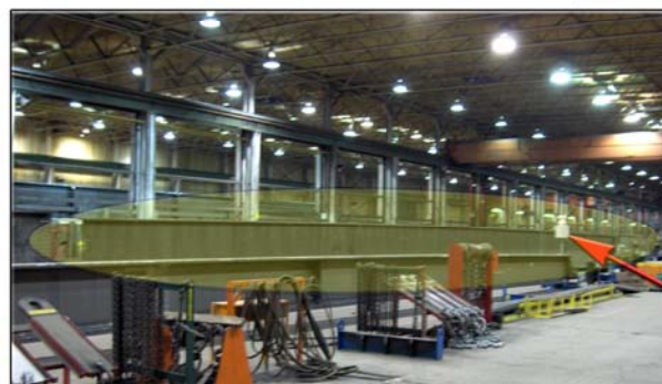
Measure large objects: camber, sweep, length
