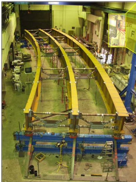
FHWA Curved Girder Bridge TFHRC Structures Laboratory
