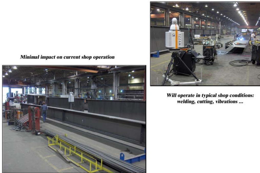
FIGURE 17 Laser system operating in a fabrication shop environment.
