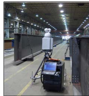
Measure girder ends: length, end-kick
