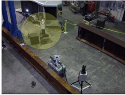
FIGURE 14 Curved girder specimen measurements of global parameters.
