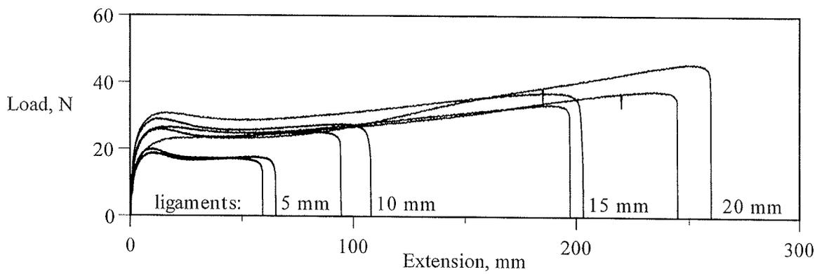
Figure 4.60 Typical duplicate measurements for essential and plastic work of fracture tests on 118-4 binder.
