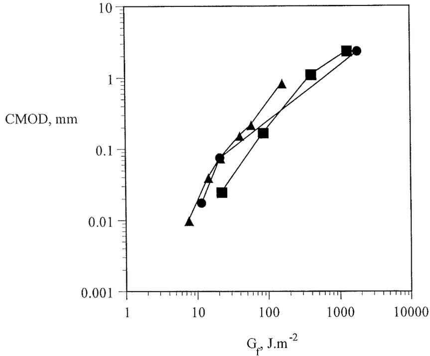
Figure 4.23 Comparisons of  $G_f$  and CMOD in the brittle and ductile regimes for 118-1 (PAV (▲)) and 118-4 (PAV (■) and recovered (●)) section binders.
