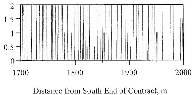
Figure 4.30 Transverse crack map for section BB (PG 52-28) on Highway 631.
