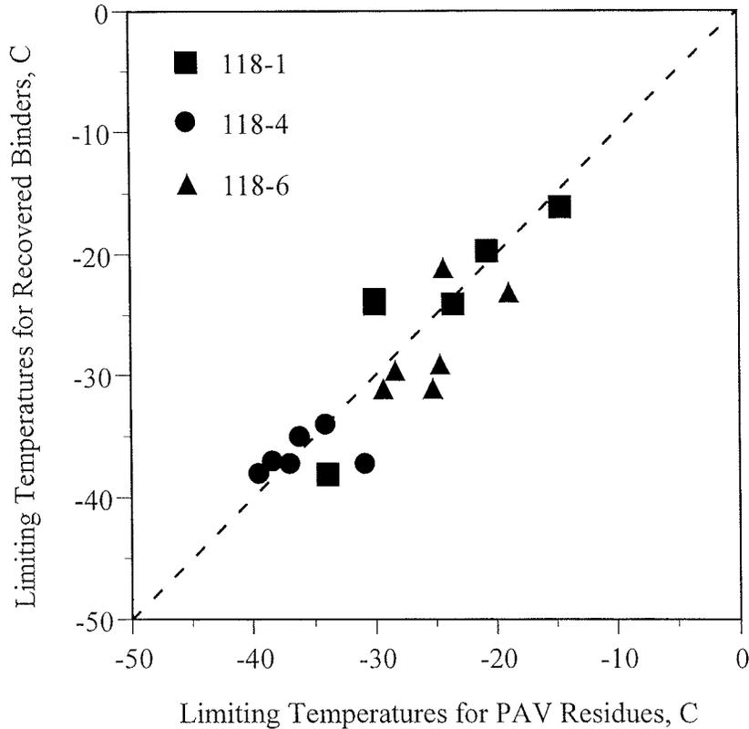
Figure 4.3 Comparison of limiting S, m and MP1a temperatures obtained on PAV residues with those obtained on recovered samples.
