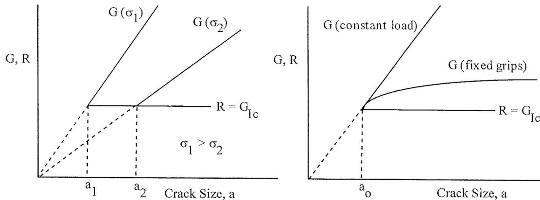
Figure 4.12 Graphical representation of the energy balance approach for plane strain fracture.  $G$  = strain energy release rate;  $R$  = resistance to fracture;  $\sigma_1$  and  $\sigma_2$  are stress levels;  $G_{Ic}$  = plane strain fracture energy. (Reproduced from Ewalds and Wanhill (1985))
