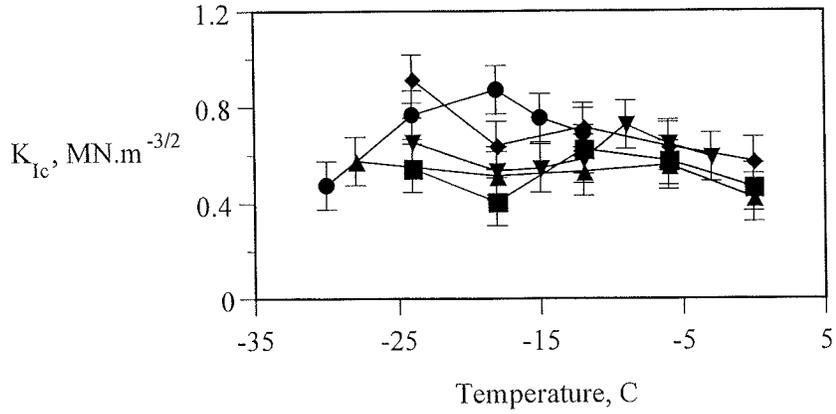
Figure 4.53 Mixture Fracture Toughness Data for Highway 118 Materials.
