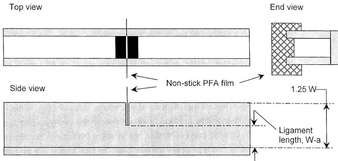
Figure 6 SENB mold assembly for specimen preparation.
