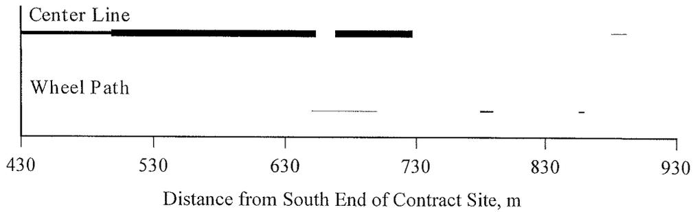
Figure 4.32 Longitudinal crack map for section A (PG 52-28) on Highway 631.
