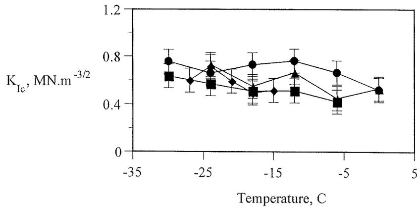
Figure 4.56 Mixture Fracture Toughness Data for Highway 17 Materials. (▲ – 17-4 (PG 58-28), ■ – 17-5 (PG 58-34 NP), ● – 17-3 (PG 58-34 P), ◆ – 17-2 (PG 58-40))
