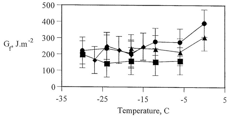
Figure 4.57 Mixture Fracture Energy Data for Highway 17 Materials. (▲ – 17-4 (PG 58-28), ■ – 17-5 (PG 58-34 NP), ● – 17-3 (PG 58-34 P), ◆ – 17-2 (PG 58-40))
