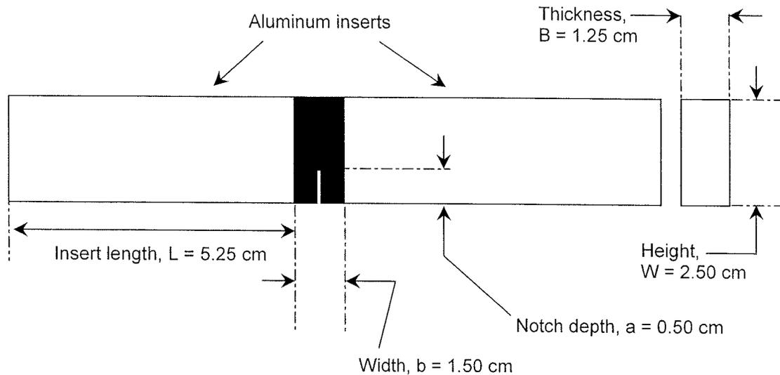
Figure 3 SENB specimen geometry.
