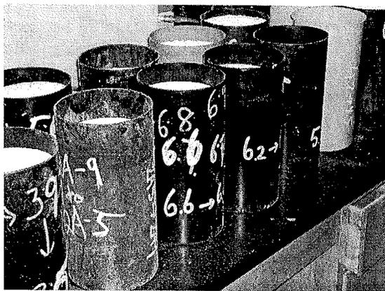
Figure 3.1 Tubes used for securing field core samples during transportation and storage.
