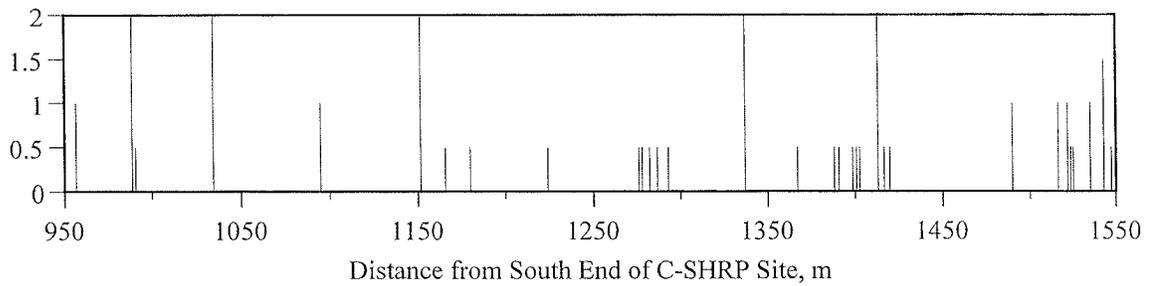
Figure 4.29 Transverse crack map for section AA (PG 46-34) on Highway 631.
