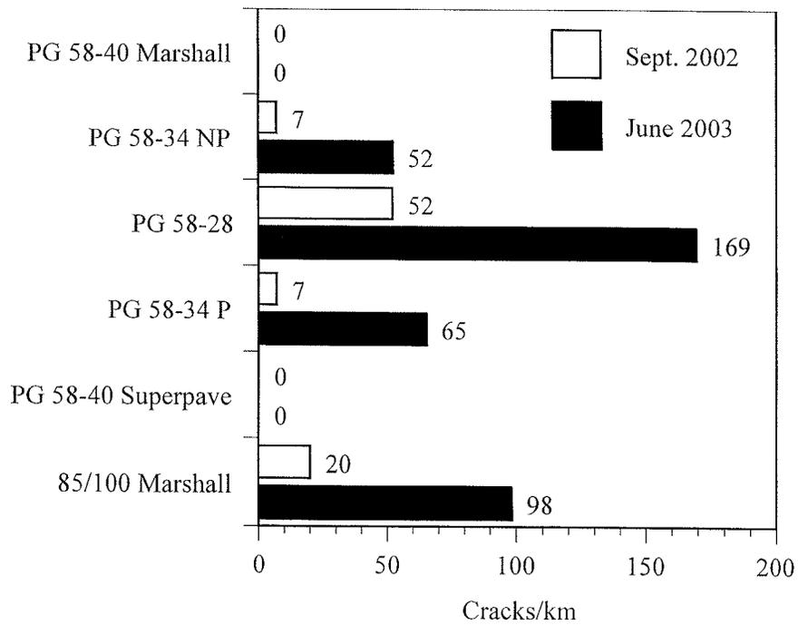
Figure 4.47 Summarized crack data for Highway 17 test sections.
