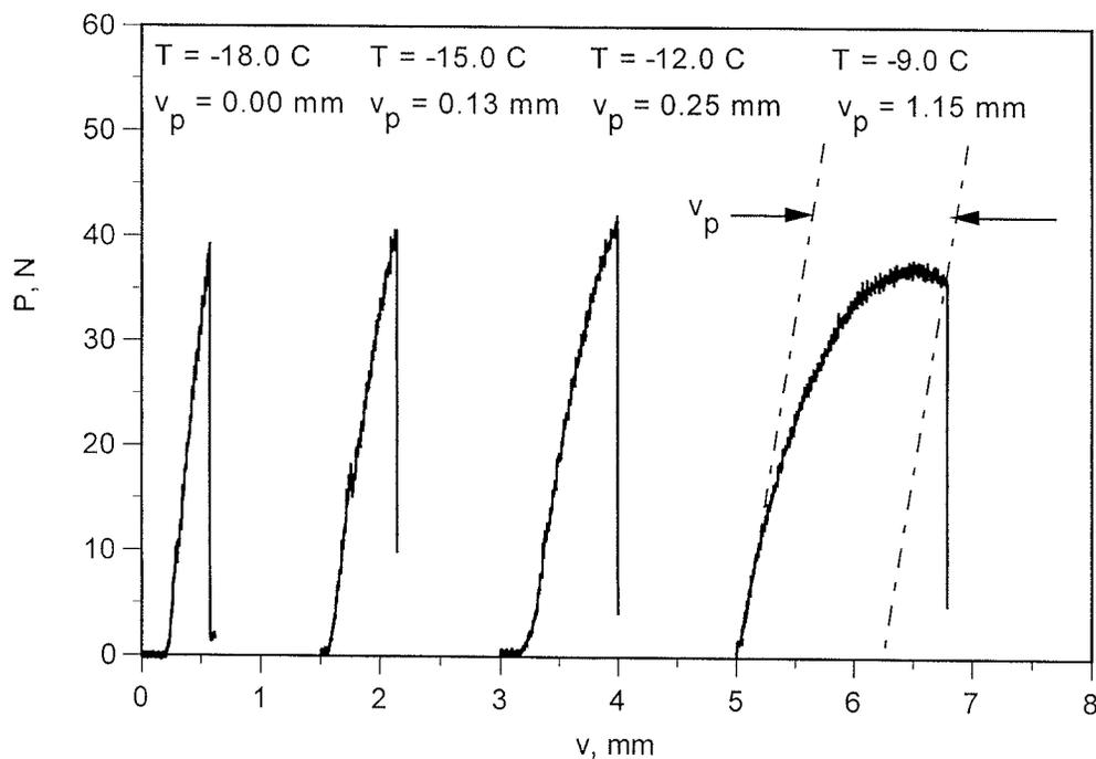
**Figure 7 Typical load-displacement curves in SENB grading tests.**
