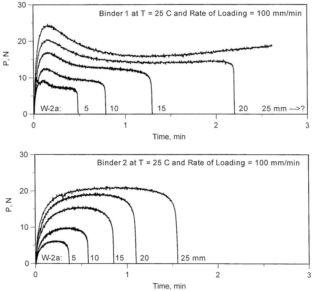
Figure 9 Typical load-displacement curves for essential work of fracture testing of two modified binders that individually show self-similar behavior yet differ between each.
