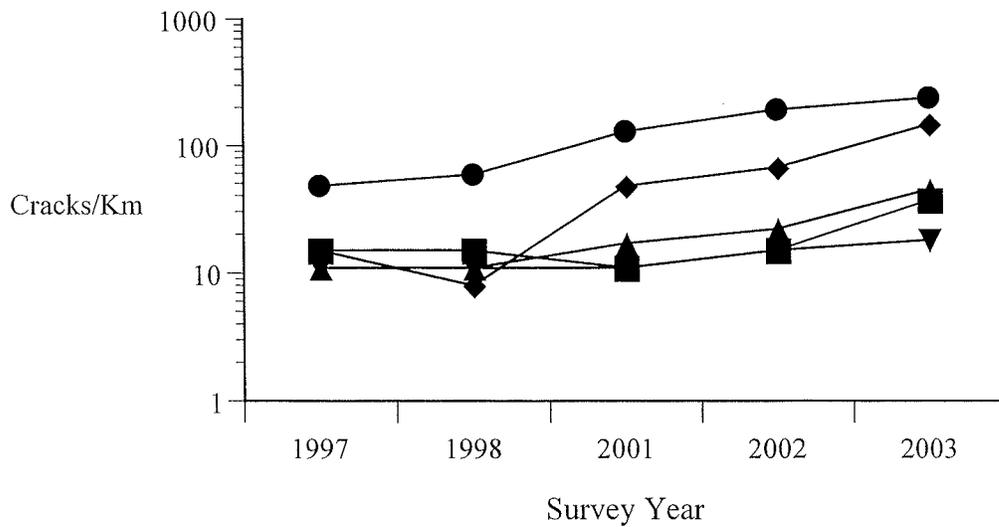
Figure 4.40 Historical crack data for Highway 118 sections 1 (●), 3 (▲), 4 (▼), 5 (■) and 6 (◆).
