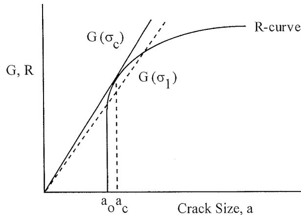
Figure 4.13 Graphical representation of a rising R-curve and stable crack growth.  $G$  = strain energy release rate;  $R$  = resistance to fracture;  $\sigma_1$  and  $\sigma_2$  are stress levels;  $a_0$  = crack size where stable crack growth starts;  $a_c$  = crack size at which catastrophic failure occurs.
