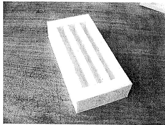
Figure 4.16 Alternative method for casting specimens with or without inserts ( $W = 25.4$  mm,  $B = 12.7$  mm,  $45^\circ$  angle,  $a = 12.7$  mm).
