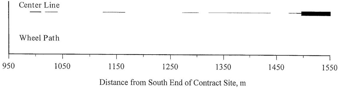
Figure 4.33 Longitudinal crack map for section AA (PG 46-34) on Highway 631.
