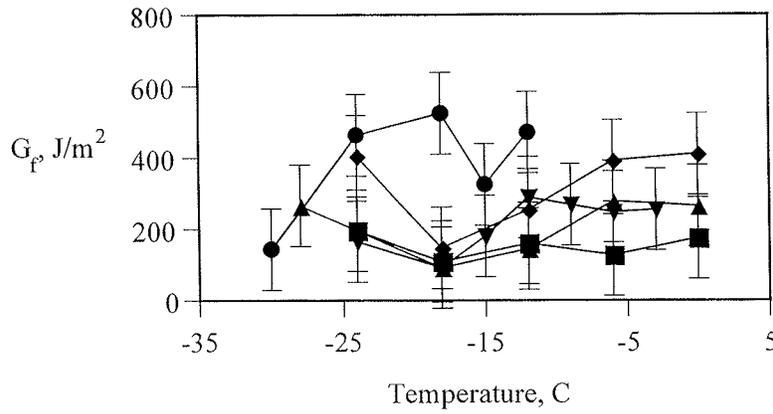
Figure 4.54 Mixture Fracture Energy Data for Highway 118 Materials.
