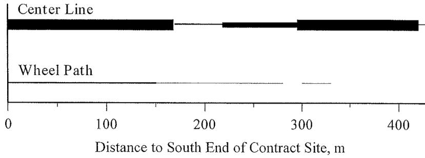
Figure 4.31 Longitudinal crack map for section B (PG 52-28) on Highway 631.
