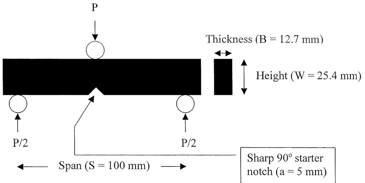
Figure 4.14 Schematic of the original fracture toughness test method (not to scale).
