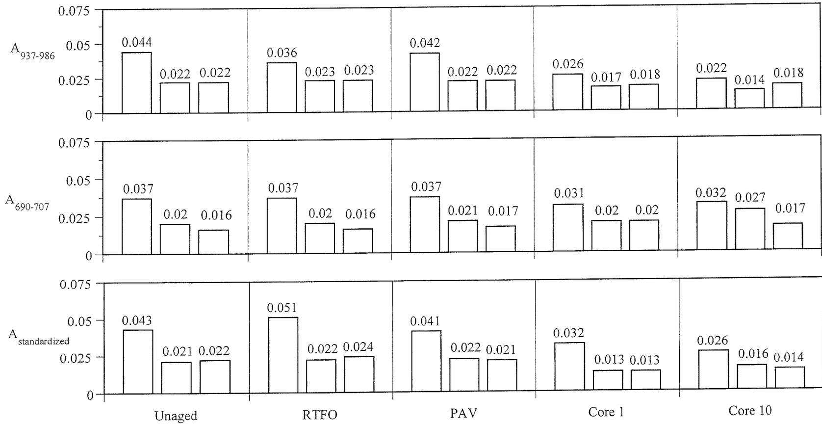
Figure 4.1 Infrared peak height data for binders from sections 118-3, 118-4, and 118-5, respectively. (The first series is for the butadiene absorbance, the second for the styrene, and the third for the butadiene corrected for variations in styrene peak height.)
