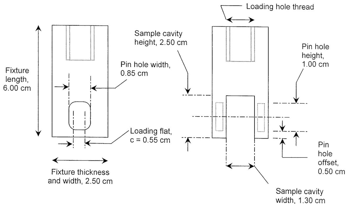
Figure 2 Clevis design for CT test.
