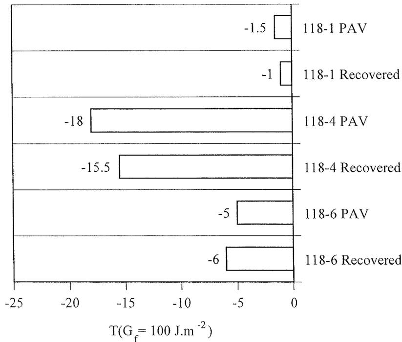
Figure 4.21 Comparisons of limiting fracture energy temperatures for 118-1, 118-4, and 118-6 section binders (not shifted).
