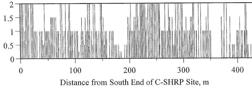
Figure 4.27 Transverse crack map for section B (PG 52-28) on Highway 631.
