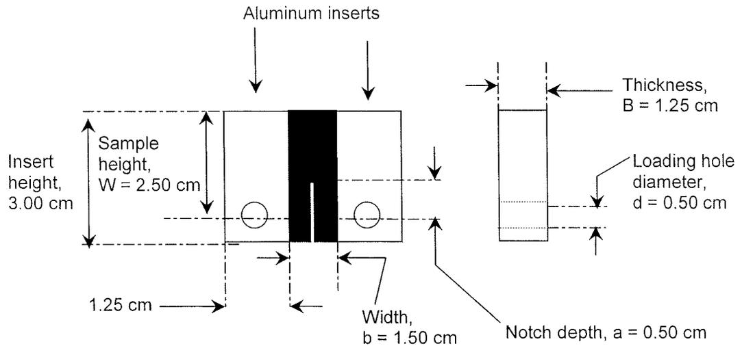
Figure 4 CT specimen geometry.
