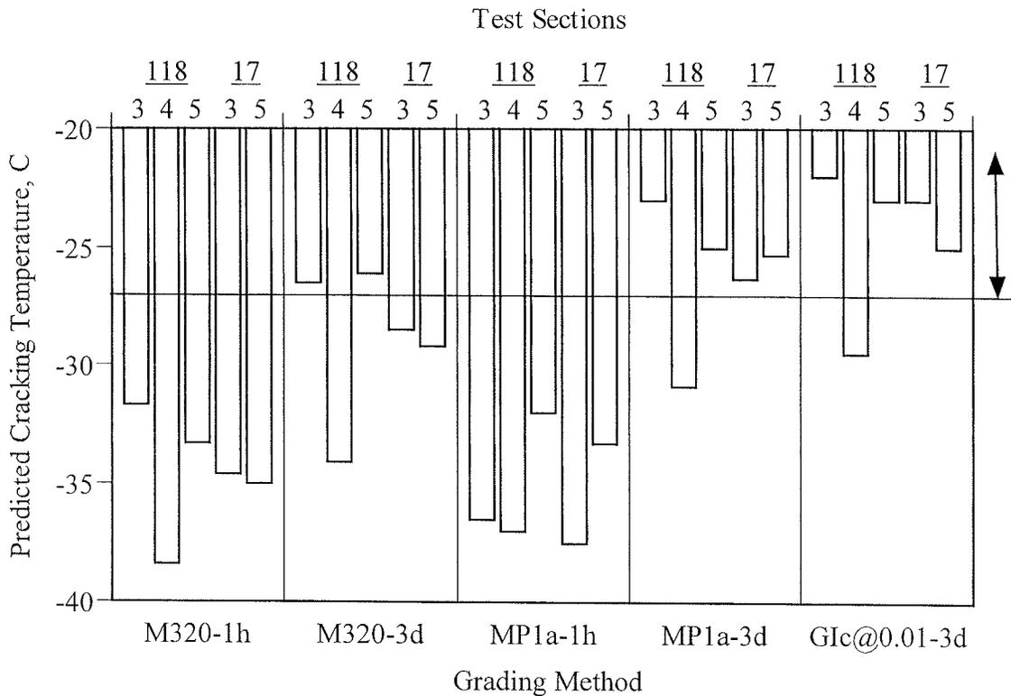
Figure 4.52 Lowest observed pavement surface temperatures compared to predicted cracking temperatures for sections 118-3, 118-4, 118-5, 17-3 and 17-5: M320-1h – AAHTO M320 after one-hour soak; M320-3d – AASHTO M320 after three-day soak; MP1a-1h – MP1a after one-hour soak; MP1a-3d – MP1a after three-day soak; and G1c@0.01-3d – limiting  $G_{Ic} = 100 \text{ J/m}^2$  @ 0.01 mm/s temperature after three-day soak.
