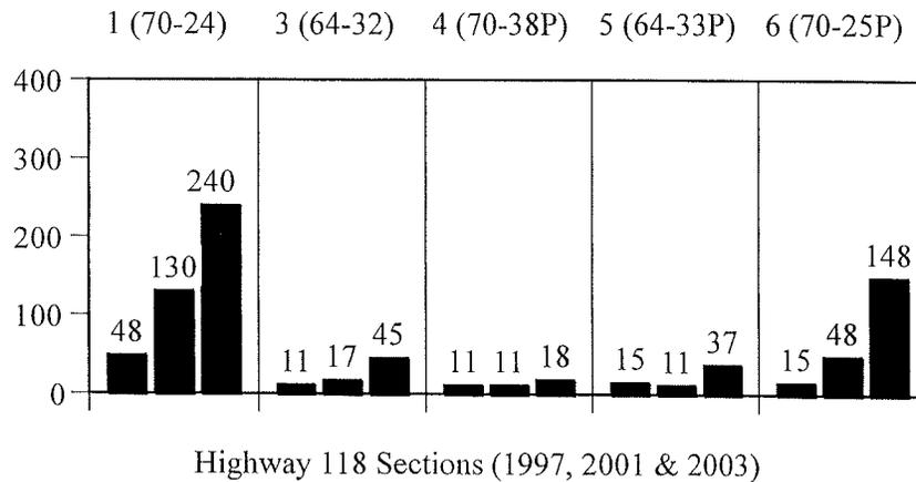
Figure 4.50 Historical cracking data for Highway 118 sections.
