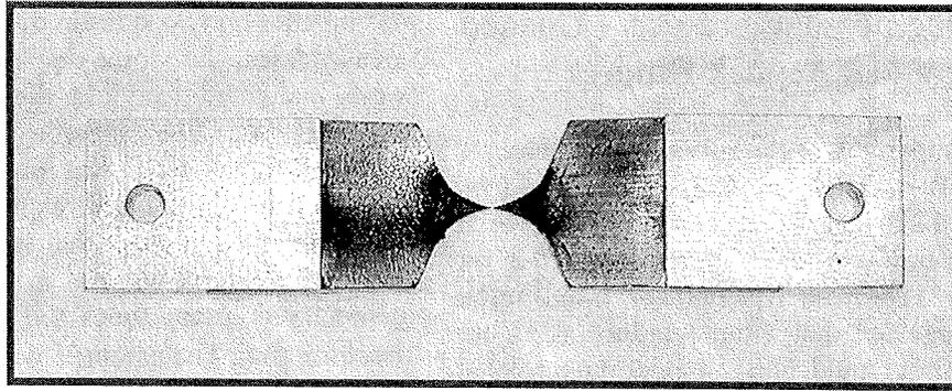
Figure 4.59 Typical DENT specimen after testing in the essential work of fracture method.
