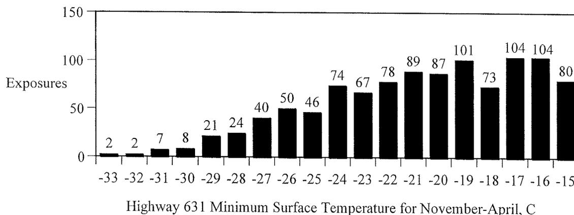
Figure 4.24 Minimum pavement surface temperatures for Highway 631 test sections as calculated from air temperatures recorded at the nearest weather station in Kapuskasing.
