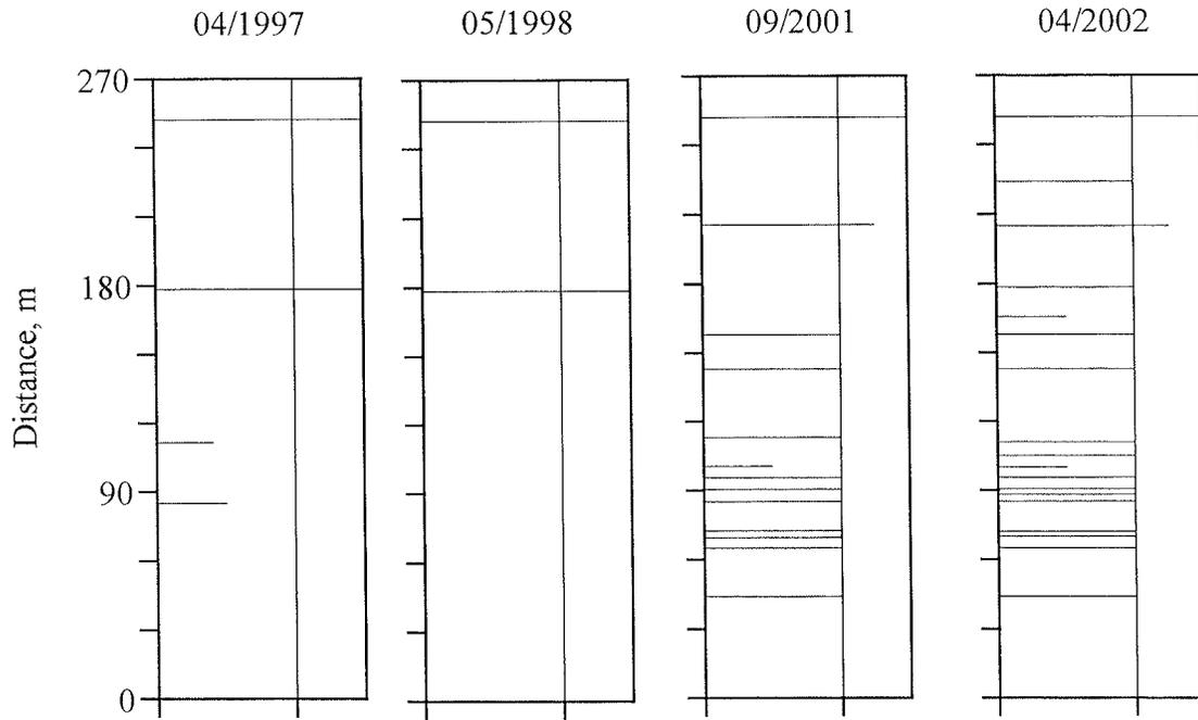
Figure 4.39 Crack maps for section 118-6.
