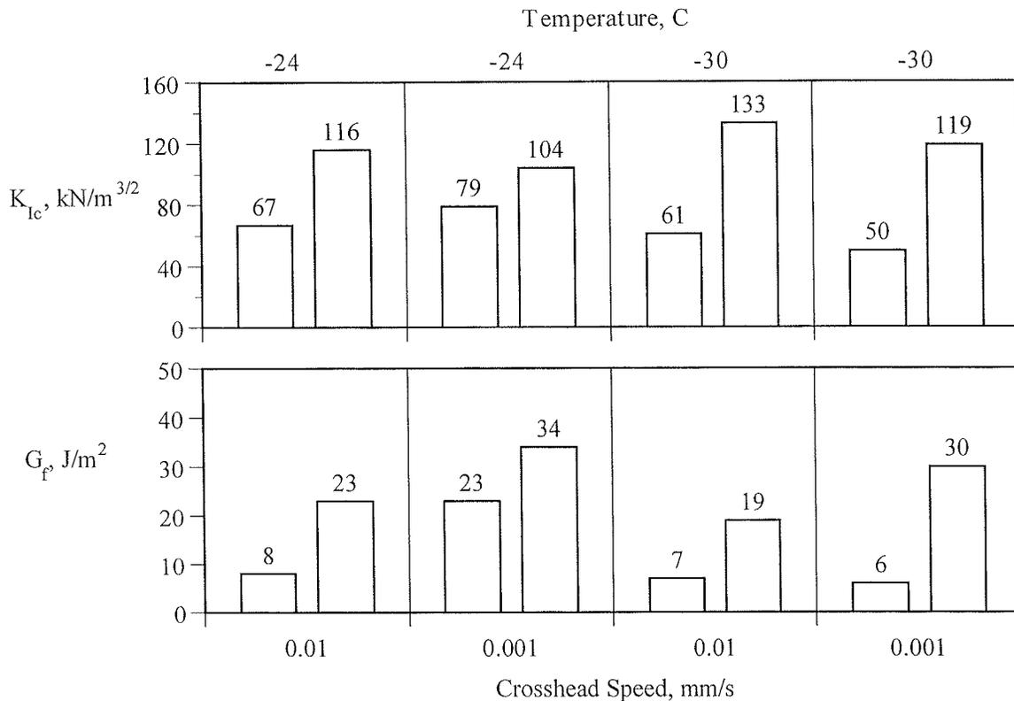
Figure 4.20 Comparison of binder fracture data for sections 118-1 and 118-6, respectively.
