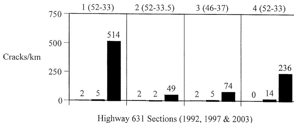
Figure 4.49 Historical cracking data for Highway 631 C-SHRP sections.
