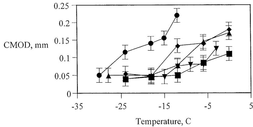
Figure 4.55 Mixture Crack Mouth Opening Displacement Data for Highway 118 Materials.
