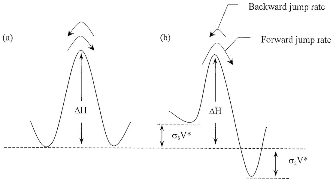
Figure 4.5 Schematic of the flow process as described by Eyring. (a) Before stress is applied with equal jump rates. (b) After stress is applied with segments preferentially jumping in the forward direction. (Reproduced from McCrum et al. (1997))
