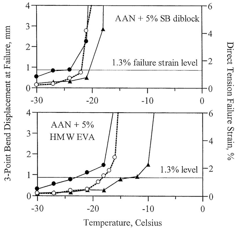
Figure 2.2 Effect of notching on the ductile-brittle transition in two modified binders. (Reproduced from Hoare and Hesp (2000))
