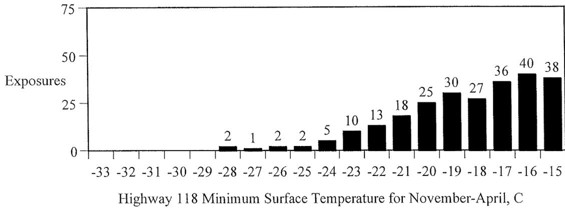
Figure 4.25 Minimum pavement surface temperatures for Highway 118 test sections as calculated from air temperatures recorded at the nearest weather station in Muskoka.
