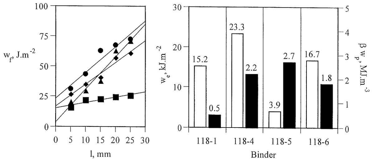
Figure 4.61 Essential works of fracture and plastic works of fracture terms at 0°C and 30 mm/min for (■) 118-1, (●) 118-4, (▲) 118-5, and (◆) 118-6 binders.
