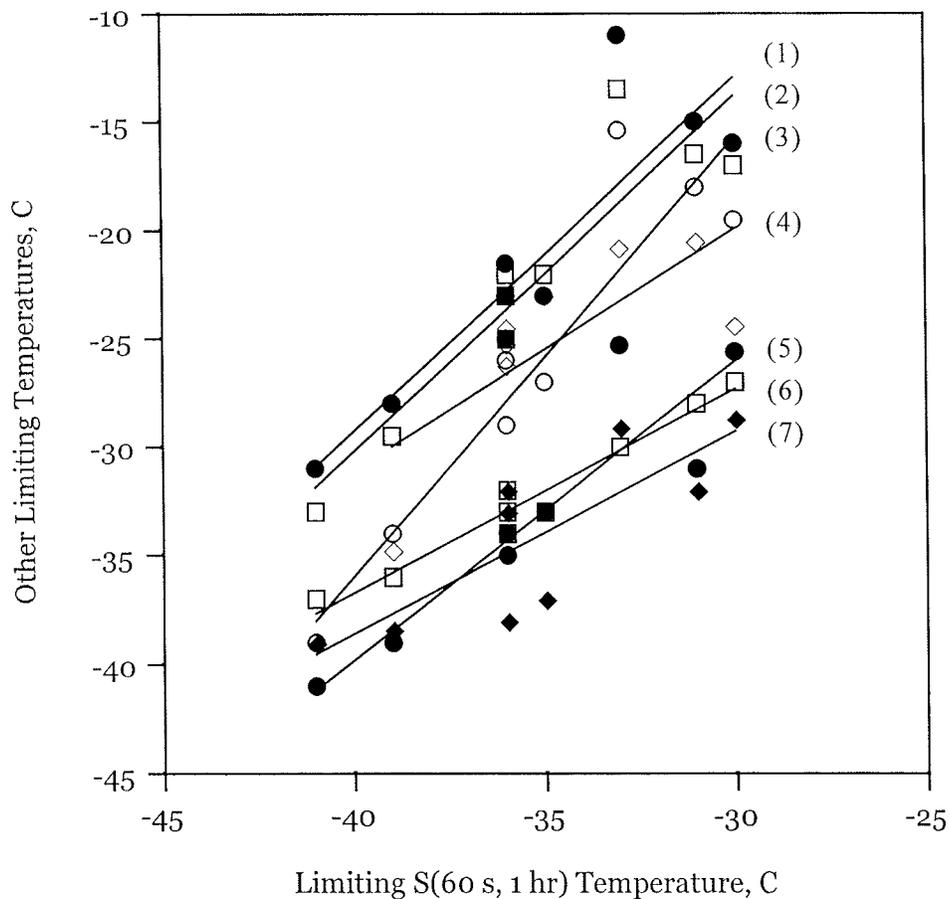
Figure 4.48 Comparisons of limiting temperatures: (1) ● –  $G_{Ic} = 100 \text{ J/m}^2 @ 0.01 \text{ mm/s}$ ; (2) □ –  $G_{Ic} = 100 \text{ J/m}^2 @ 0.001 \text{ mm/s}$ ; (3) ○ –  $m(60 \text{ s}) = 0.3$  after three-day soak; (4) ◇ – MP1a after three-day soak; (5) ● –  $m(60 \text{ s}) = 0.3$  after one-hour soak; (6) □ –  $S(60 \text{ s}) = 300 \text{ MPa}$  after three-day soak; and (7) ◆ – MP1a after one-hour soak.
