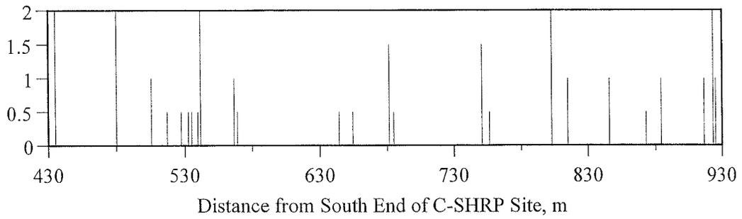
Figure 4.28 Transverse crack map for section A (PG 52-28) on Highway 631.
