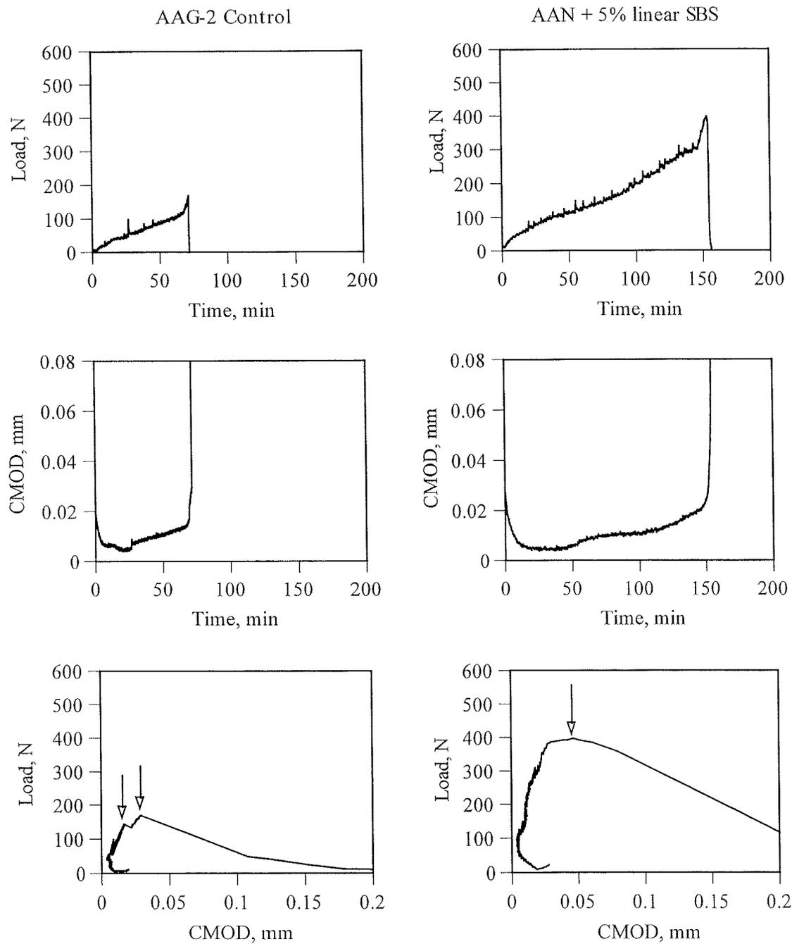
Figure 4.10 Representative crack mouth opening displacement results for AAG-2 control and AAN + 5% linear SBS mixtures at  $-30^{\circ}\text{C}$  and strain rate of 0.01 mm/min.
