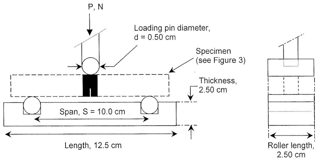
Figure 1 Bending rig for SENB test.
