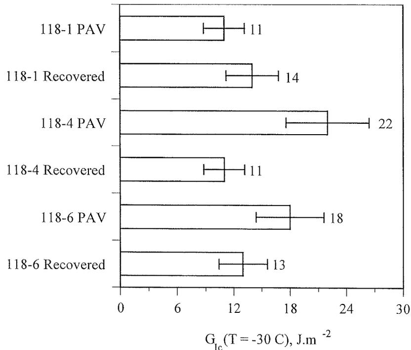
Figure 4.22 Comparisons of fracture energies in the brittle regime for 118-1, 118-4, and 118-6 section binders (estimated error bars of  $\pm 20$  percent).
