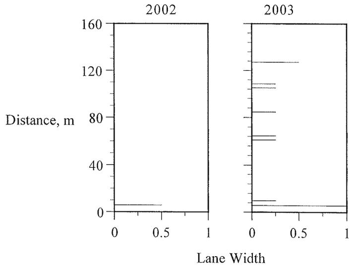
Figure 4.46 Crack maps for section 17-3 (PG 58-34 NP).
