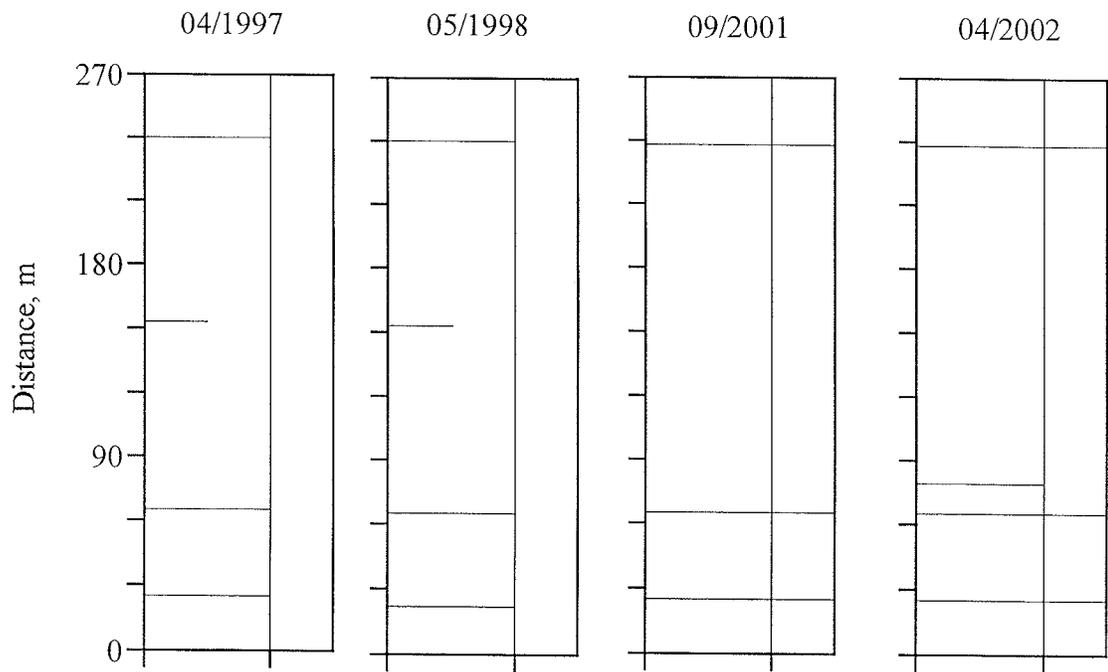
Figure 4.38 Crack maps for section 118-5.
