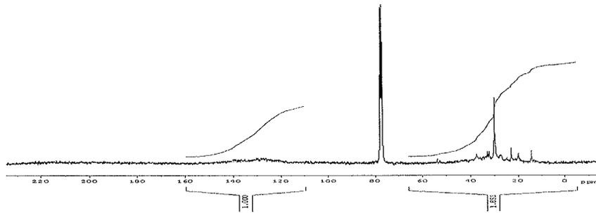
Figure 3.5 Typical  $^{13}\text{C}$  NMR spectrum for binder from section 3 on Highway 118.
