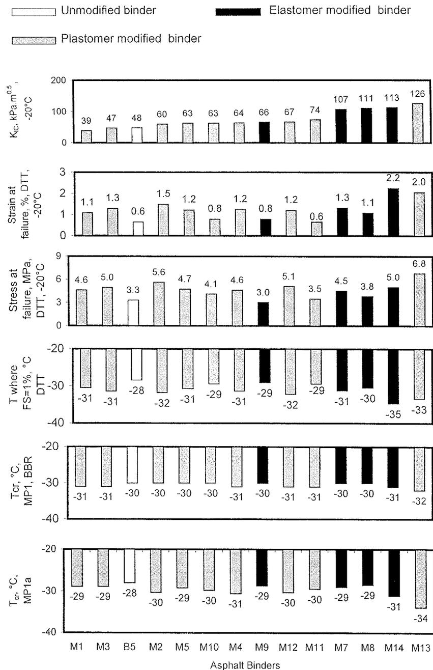
Figure 2.4 Low-temperature specification data in contrast with fracture toughness for a range of straight and modified asphalt binders. (Reproduced from Anderson et al. (2001))
