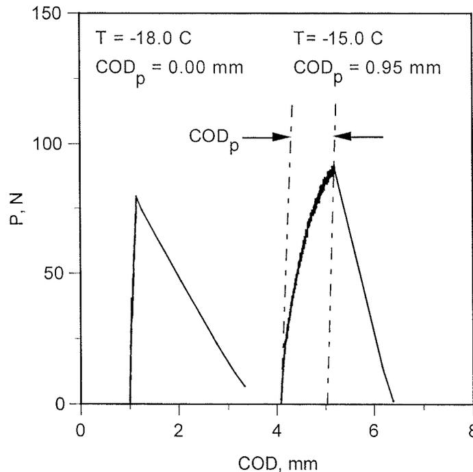
Figure 8 Typical load-crack opening displacement curves in SENB grading tests.
