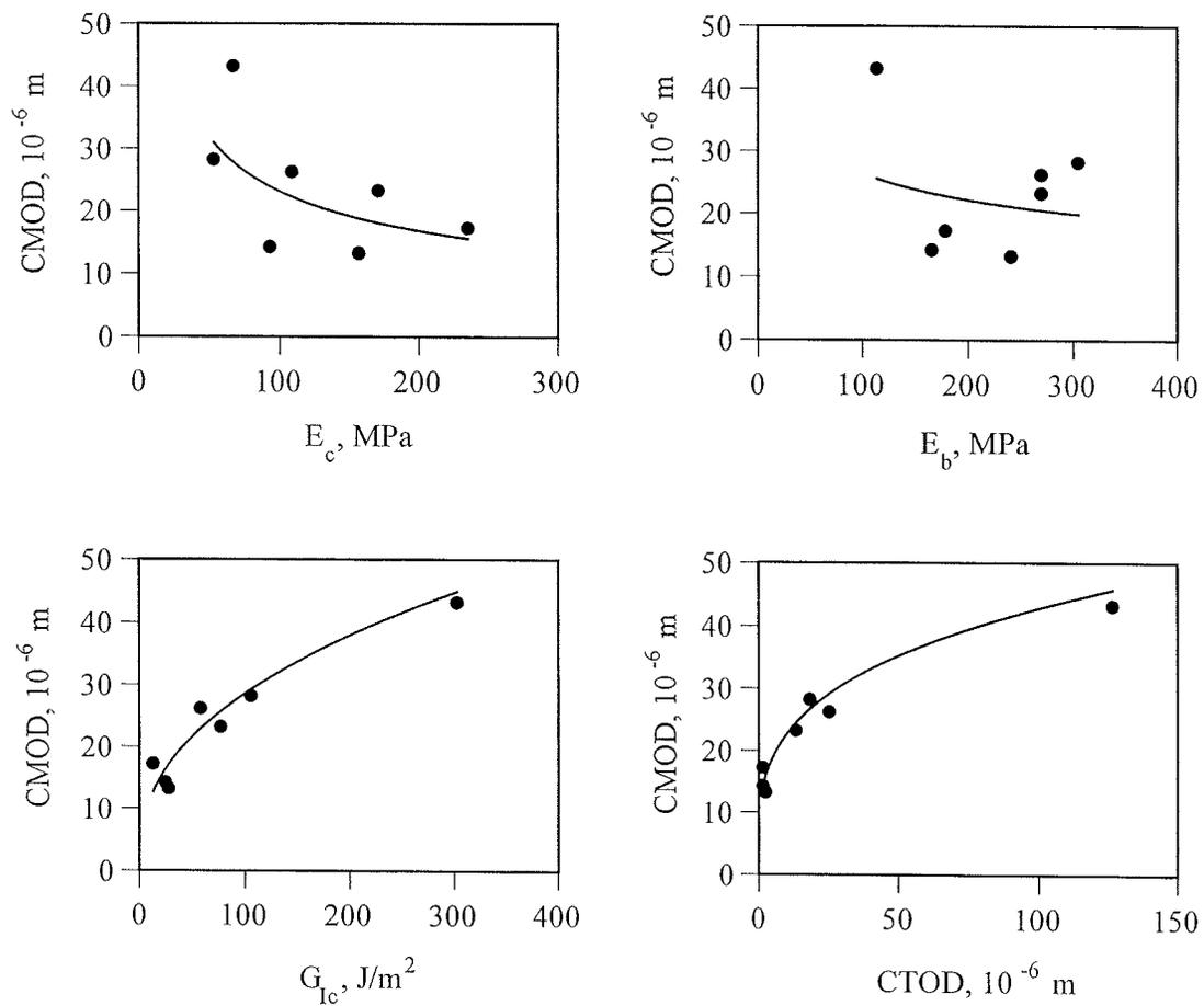
Figure 4.11 Correlation between mixture CMOD and various binder properties.
