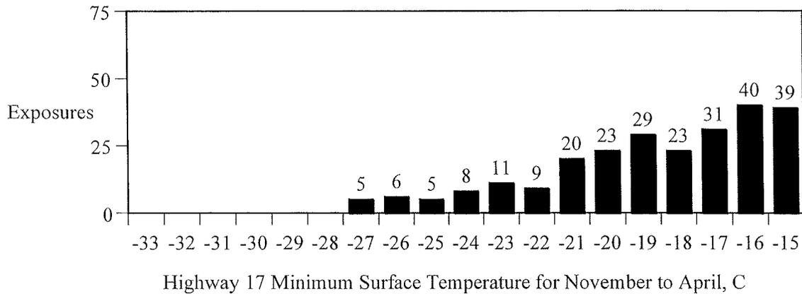
Figure 4.26 Minimum pavement surface temperatures for Highway 17 test sections as calculated from air temperatures recorded at the nearest weather station at CFB Petawawa.
