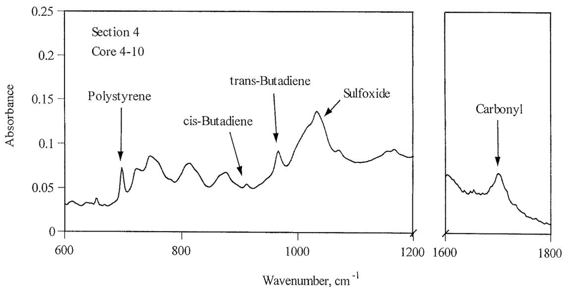
Figure 3.3 Infrared spectrum for a binder sample from section 4 on Highway 118.
