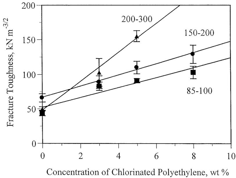
Figure 2.1 Effect of polymer concentration and bitumen grade and source on fracture toughness in chlorinated polyethylene systems (error bars give 90 percent confidence level). (Reproduced from Lee et al. (1995))
