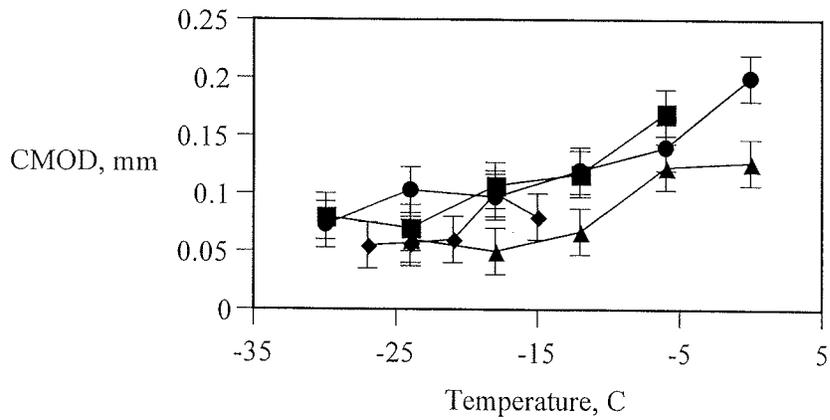
Figure 4.58 Mixture Crack Opening Displacement Data for Highway 17 Materials. (▲ – 17-4 (PG 58-28), ■ – 17-5 (PG 58-34 NP), ● – 17-3 (PG 58-34 P), ◆ – 17-2 (PG 58-40))
