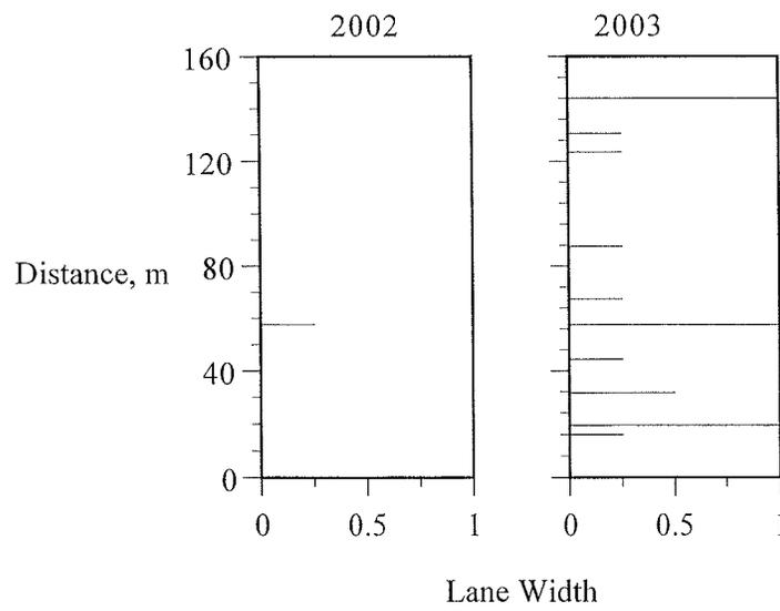
Figure 4.45 Crack maps for section 17-2 (PG 58-34 P).
