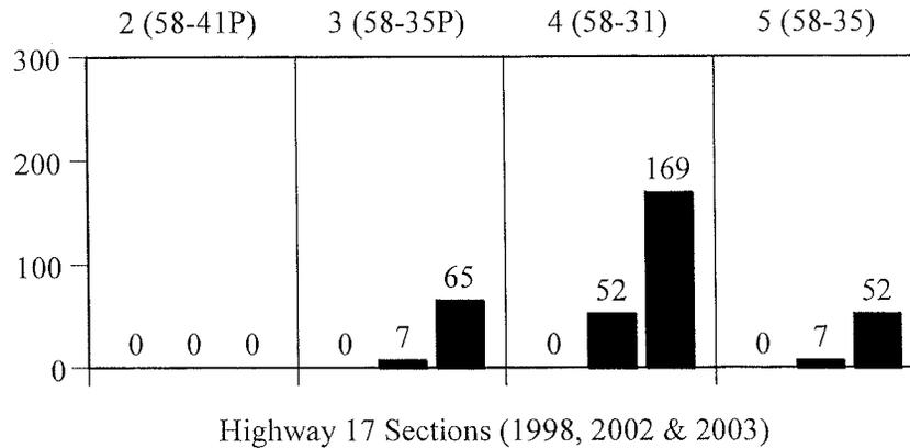
Figure 4.51 Historical cracking data for Highway 17 SPS-9A sections.
