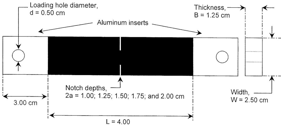
Figure 5 DENT specimen geometry.
