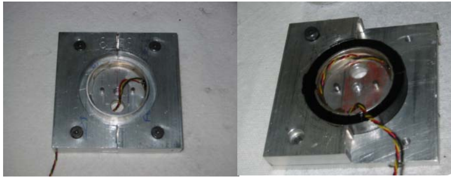
FIGURE 4.2 Aluminum molds (left), aluminum mold with a trimmed binder specimen.
