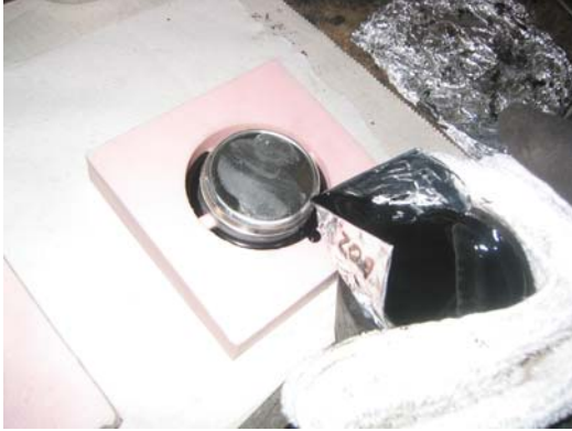
FIGURE 4.4 Pouring sample from steel cup with aluminum foil spout.
