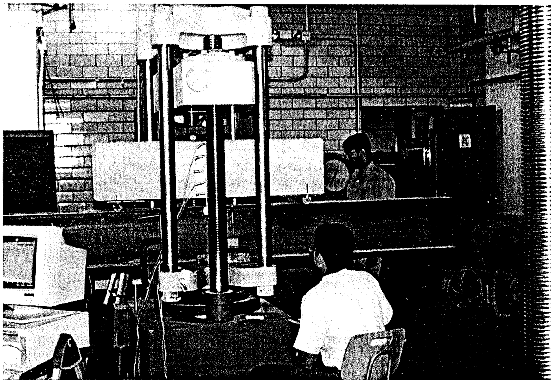
Photo 7 Test set-up for Basalt Reinforced Beam Data Acquisition Software(Mega-Dac)seen in the picture
