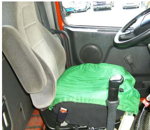
Figure 2.1-3. Air-inflated seat cushion mounted on original truck seat
