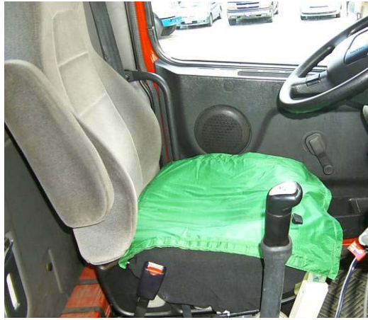
Figure 3.1-2. Air-inflated seat cushion mounted on original truck seat
