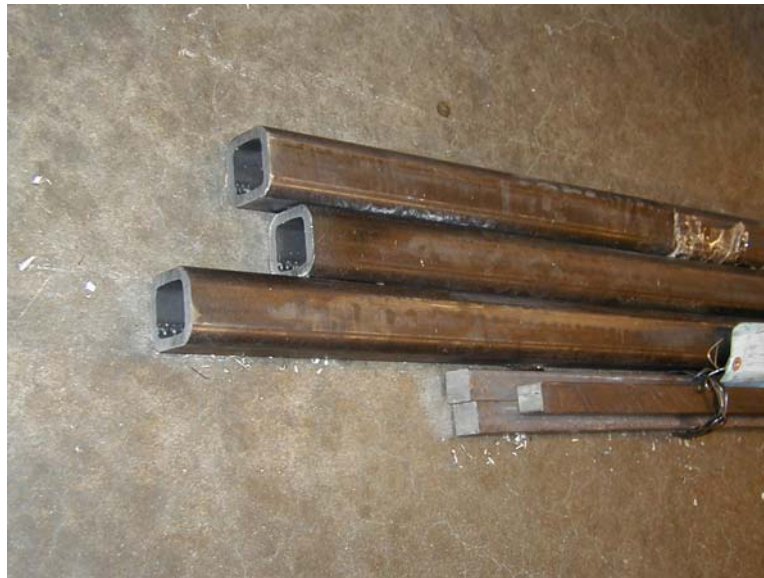
Figure 3: Sleeve (upper) and Core (lower) Pieces Used for Testing
