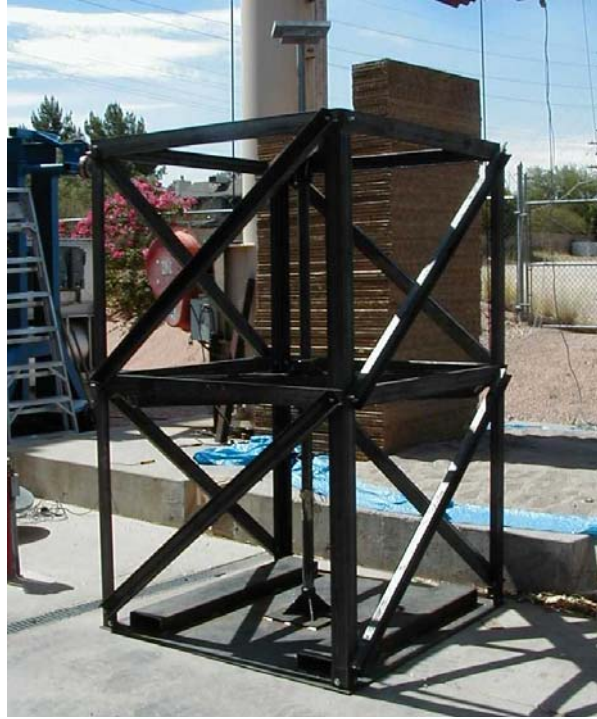
Figure 4: The Test Configuration used in Stage 2 Impact Testing; the Sleeved Column is in the Center of the Support Frame
