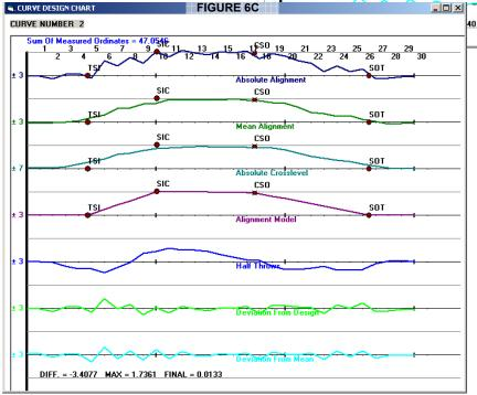
Figure 6C shows how application of the Automatic Curve Adjust (ACA) function gives a better solution (smaller throws) and the curve points are closer to the Absolute Alignment data but the DIFF is larger. By observing the deviation from design vs. the deviation from mean, either design is usable for geometry testing.
