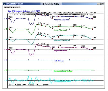
Curve 9 in Figure 13A is determined manually to be a fixed curve. The modeling of a fixed curve is established by changing the initial and final curve points to a unique pair, or by any other means, so the deviation from design is a constant zero. The curve points between the end points are not usually needed. This also demonstrates that the deviation from mean is not zero, of course, and is in fact the source of most false track geometry alignment defects.
