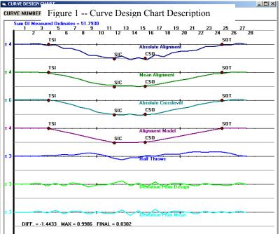
otherwise were elusive or impossible, especially on long curves. It was discovered that the curve body design was not constant over long curves. This is now obvious to the investigation that no curve body has absolutely uniform curvature. Therefore very minor adjustments of the curvature in the curve body had to be provided for. Curve points are therefore added automatically during data acquisition on each long curve body. Provision is made for adding curve points manually wherever desired.
