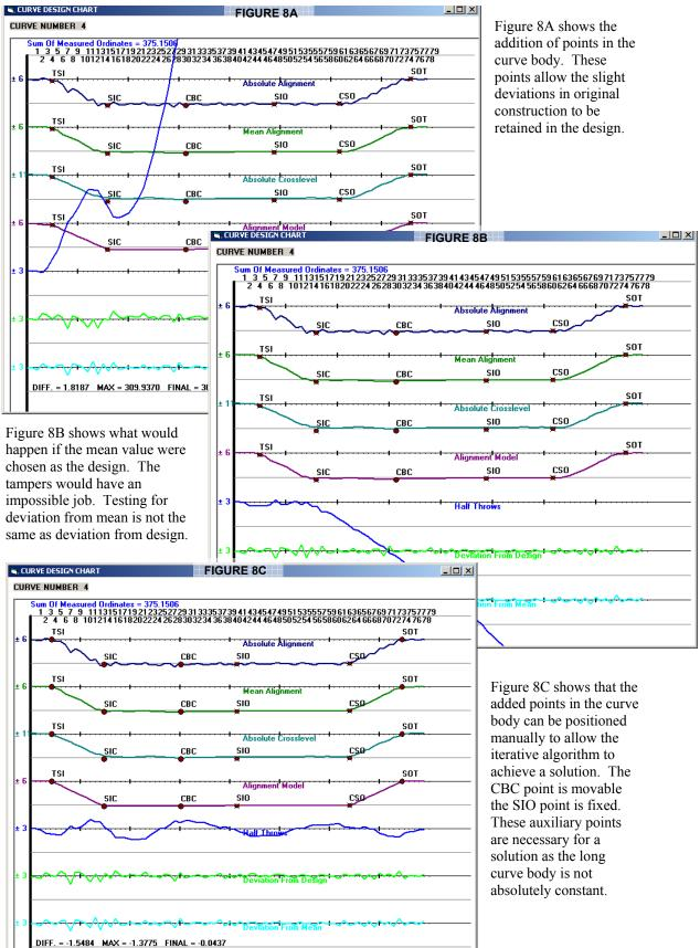
Figure 8 -- Curve 4 – Curve Points Must Be Added
