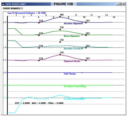
Curve 1 is also a fixed curve. Curve 9 is in a tunnel on direct fixation and Curve 2 is a turnout or switch. Both are handled such that the data acquisition serves to establish the foot-by foot shape for the database.
