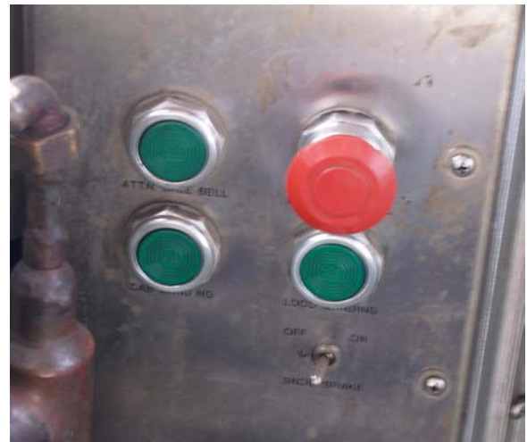
Fig 5 - Cab sand button (lower left) and loco sand button (right)
