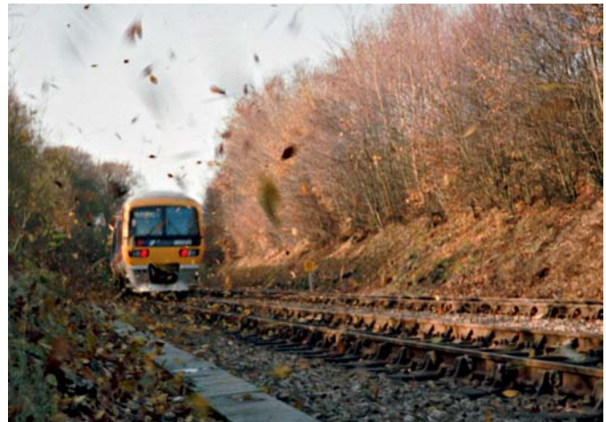
Fig. 1 - Fall Leaf Conditions Leading To Adhesion Problems
