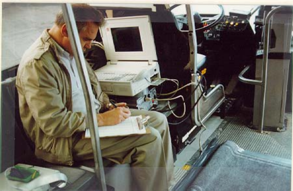
FIGURE 10 Data collection system set-up on the left front passenger seat just above the mat.
