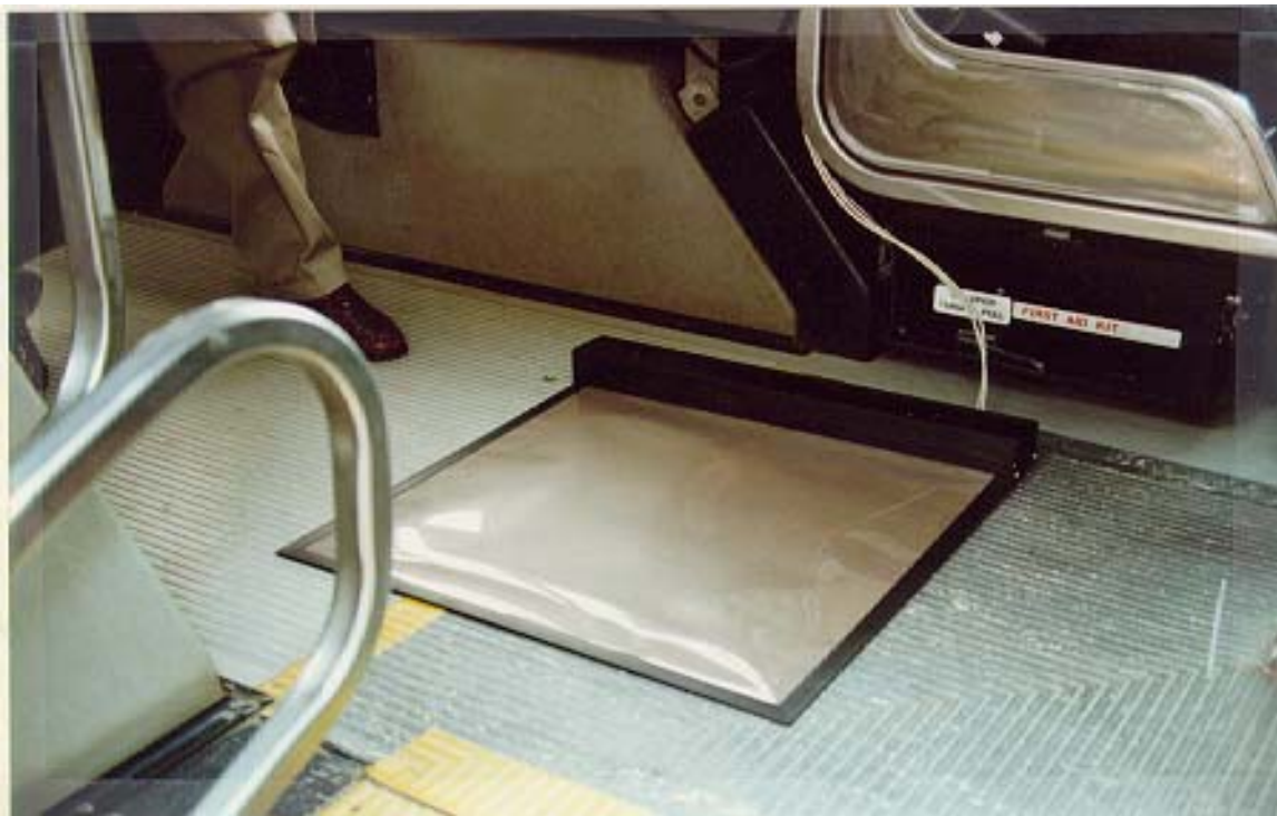
FIGURE 9 The pressure sensitive mat installed on the floor of the vehicle.
