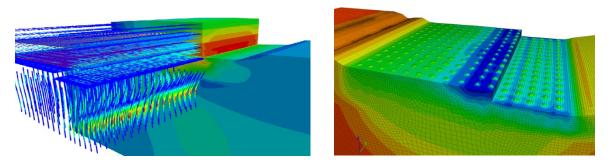
Figure 4: (a) Computer model of a column supported embankment (b) colum supports
