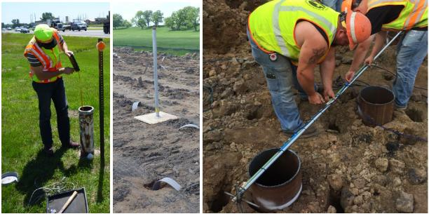
Figure 2: (a) A manual groundwater assessment using a weighted tape in a borehole piezometer; (b) a settlement plate to measure settlement in a field of prefabricated vertical drains; (c) and a series of rebar strainmeters attached to a centralizer bar before being placed in a concrete filled steel shell pile to measure strain distribution.
