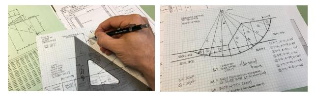
Figure 3: (a) Setting up a slope stability problem by hand (b) the finished slip surface evaluated by hand for one case using a simplified Ordinary Method of Slices evaluation.
