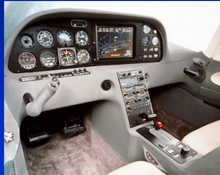
Multi-function Display Installation in General Aviation Cockpit
