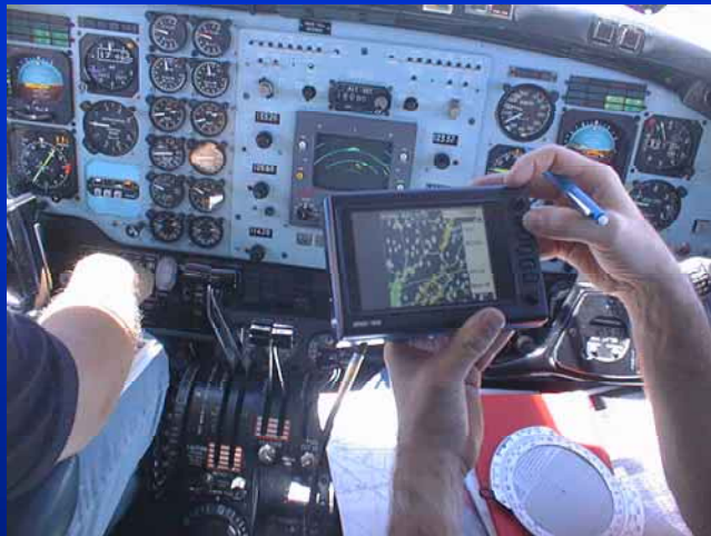
Tethered general aviation weather information system on NASA LaRC BE200 King Air
