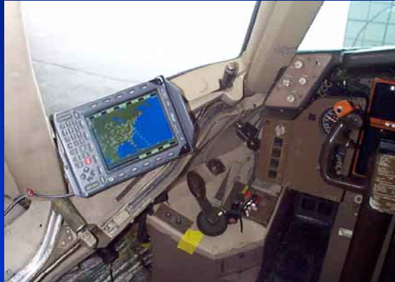
Weather Information Network (Honeywell-WINN) Avionitek Display in NASA B-757
