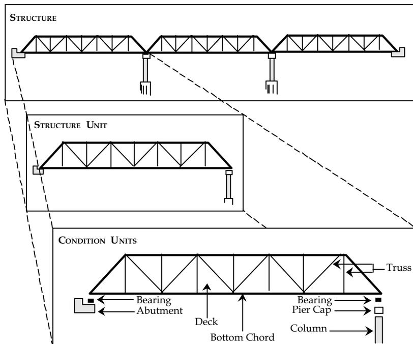
**Figure 2: Decomposition of a structure in Pontis.**
