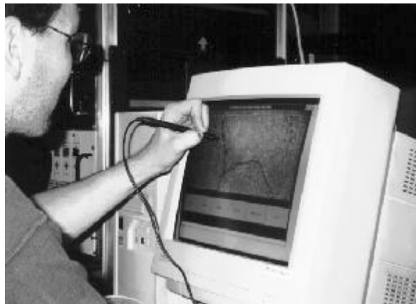
Figure 6 An Example of Human and Machine Interface Using a Touch-Sensitive Screen.
