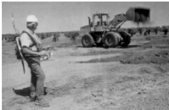
Figure 9 Teleoperated and Automated Maintenance Equipment Robotics (TAMER) System during Operation. (Hendrickson, 1995. Automation and Robotics in Highway Design, Construction, and Maintenance , TR NEWS , No. 176: 2-23.)
