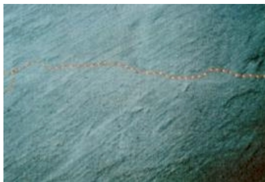
Figure 5 Crack Detection and Representation Using a Machine Vision Algorithm.
