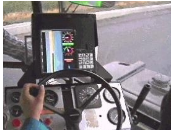
Figure 11 The onboard MMI of CIRCOM prototype during compaction.
