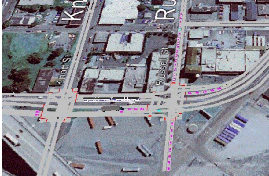
FIGURE 5 Initial traffic simulation model of Interstate Avenue at Russell Street. LRT vehicles are shown in white, buses in blue, trucks in gray, and passenger cars in pink. No train is shown on Track 100 or trucks on Russell Street.
