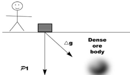
**Gravity:** Gravimeters are designed to measure variations in the gravitational field of the Earth, and are typically used to generate 2-D or 3-D density–depth models of the subsurface. If external constraints are available, the density–depth models can be transformed into a geologic model.
