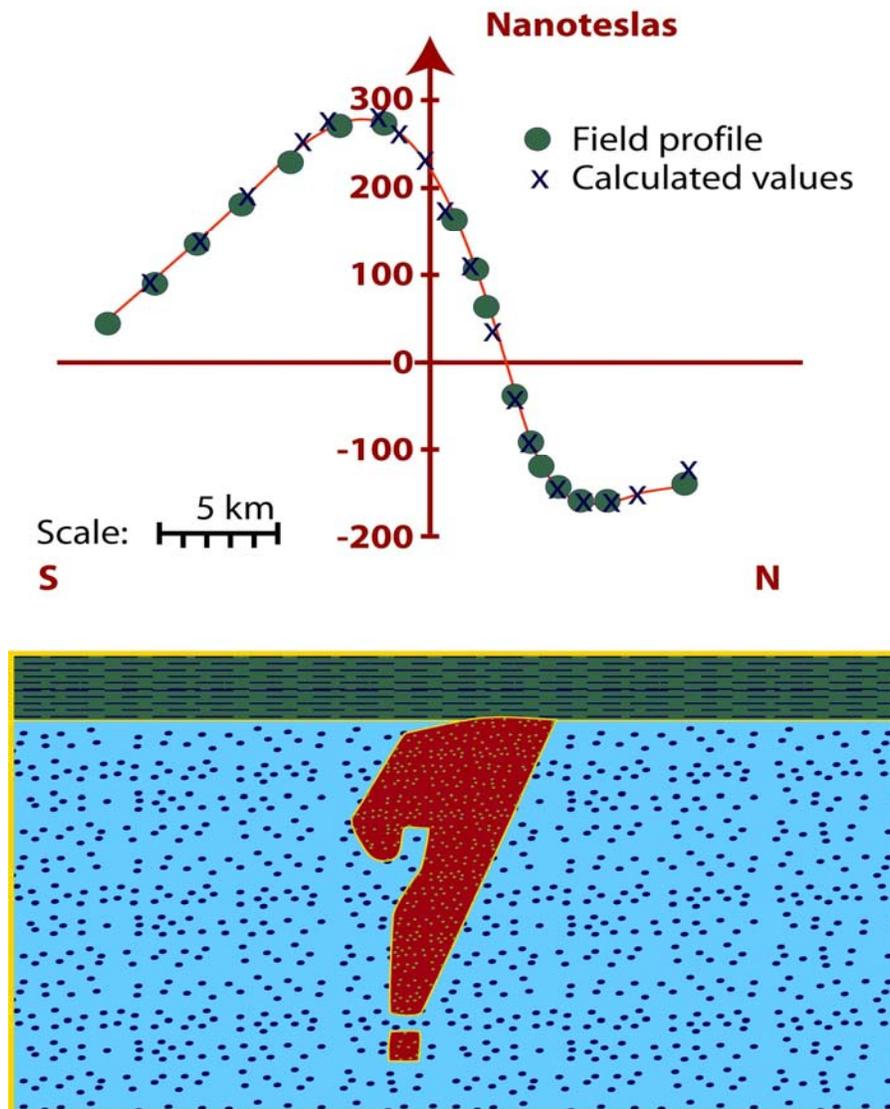
**FIGURE 6** Magnetic data acquired in Switzerland, and a corresponding subsurface interpretation that is “theoretically accurate” but geologically absurd.
