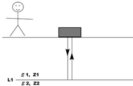
**GPR:** Typically, pulsed EM energy is generated at predetermined station locations along the length of the GPR profile. The travel times and amplitudes of reflected EM energy are usually recorded by a monostatic transmitter–receiver. The recorded travel time–amplitude information is normally used to generate a GPR profile (2-D time–amplitude image). These data can be transformed into a 2-D velocity–depth model. If external constraints are available, a geologic model can be generated.
