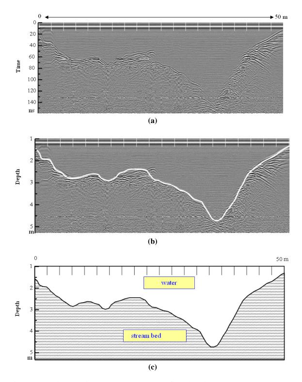
FIGURE 5 (a) GPR profile across a stream bed; (b) typical GPR physical property model (with interpreted layer boundaries); and (c) typical site model (geologic-hydrologic) (Anderson et al., 2007).
