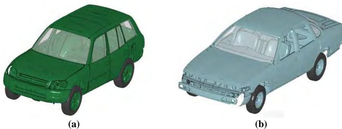
FIGURE 12 Finite element models for the additional highway vehicles used in the crash analyses: (a) HV 3, Toyota RAV4; and (b) HV 4, Ford Crown Victoria.
