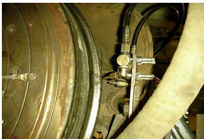
FIGURE 13 Onboard lubricator: flange lubricator on LRV117.
