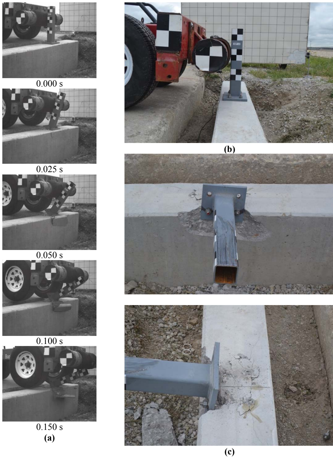
FIGURE 8 Test No. IBP-4, US-20 Bridge Anchorage: (a) sequential events; (b) pre-test; and (c) system damage.
