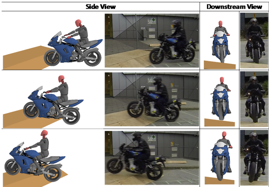
FIGURE 6 Slope tests - simulated and experimental motorcycle kinematics with 20-deg slope at 45-deg approach angle (Test 20/45-3).
