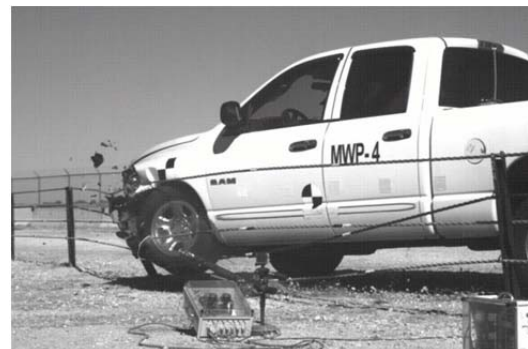
Tire overrode 1st and 3rd cable
