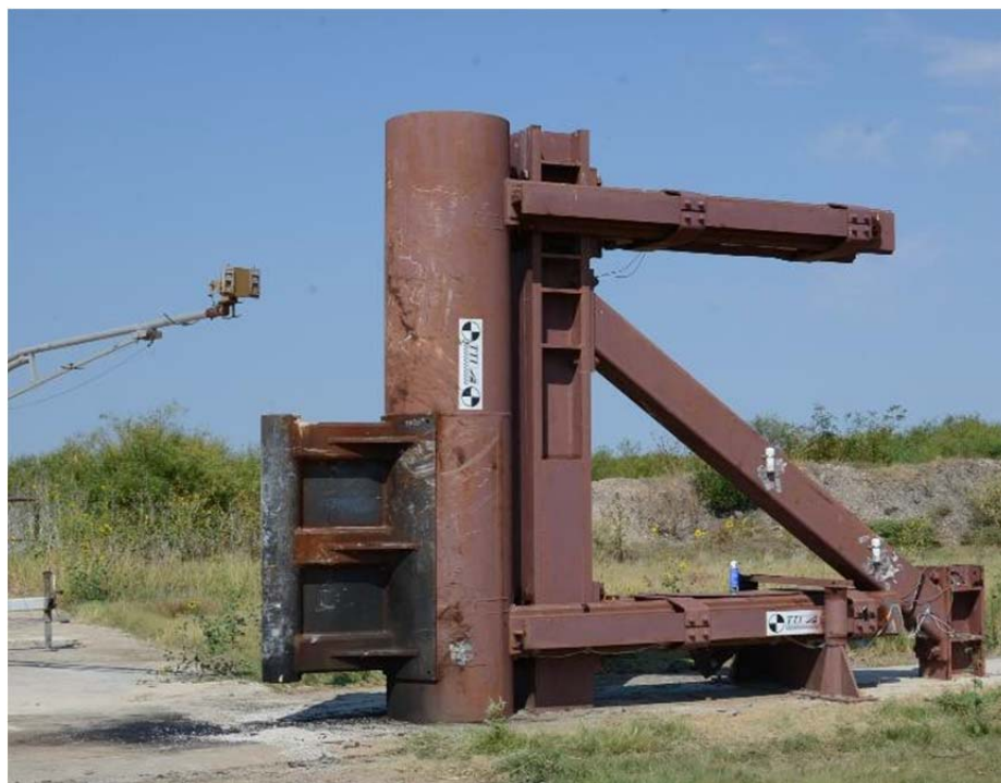
FIGURE 1 Instrumented pier and simulated bollard.
