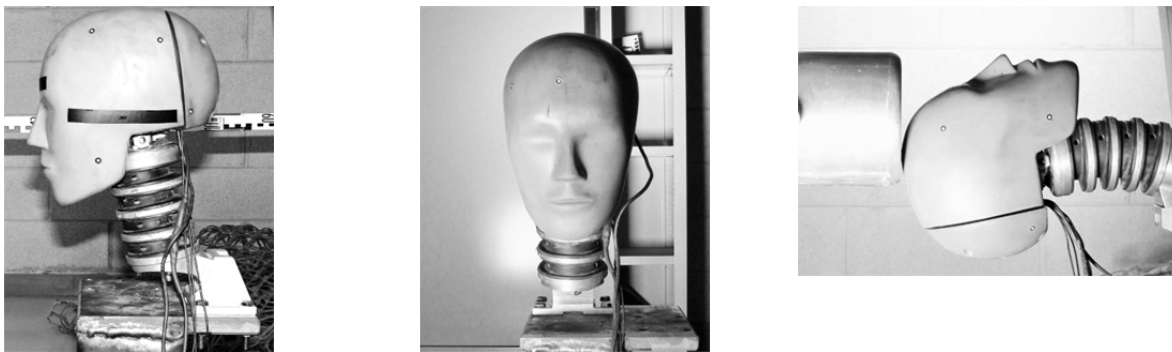
FIGURE 2 Experimental configuration for pendulum impact tests.
