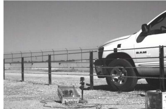
3rd cable on back side of post
