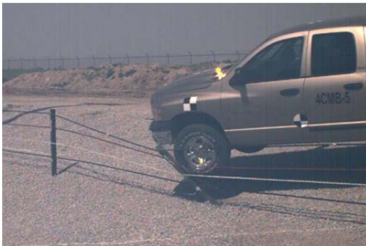
Top cable pushed down by post
