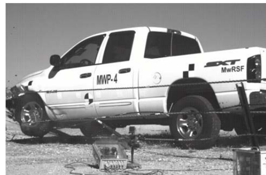
Vehicle redirected by 2nd and 4th cables
