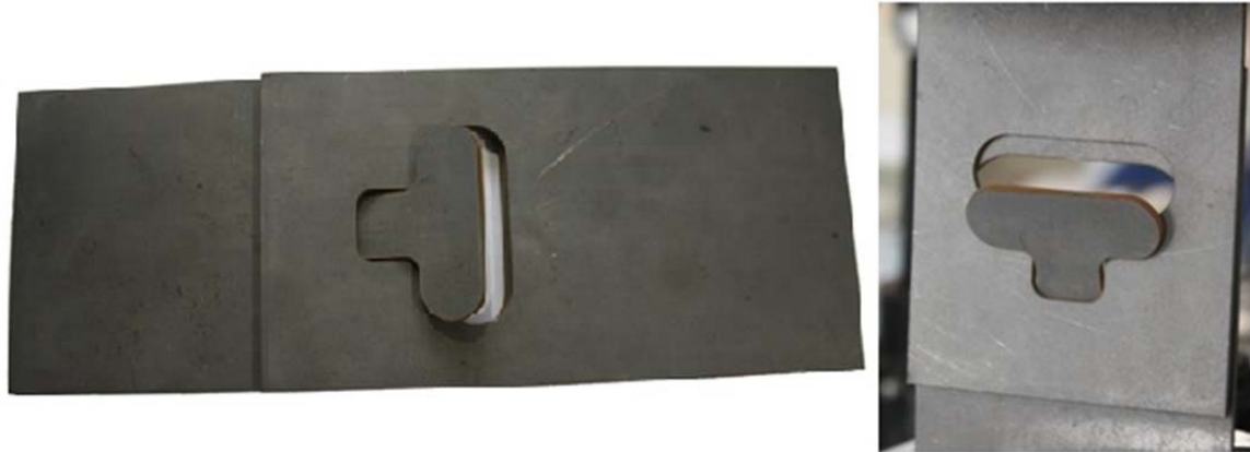
FIGURE 1 New connection, flap and hole.
