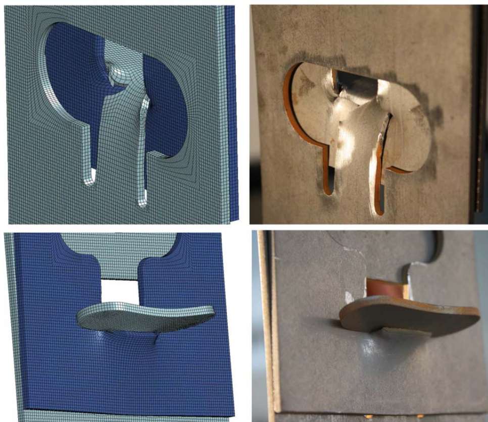
FIGURE 7 S235JR numerical-experimental qualitative comparison of tests on simplified configurations.
