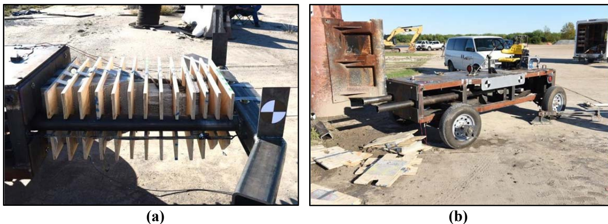
FIGURE 7 Surrogate test vehicle before and after test no. 690900-BV3: (a) before and (b) after.
