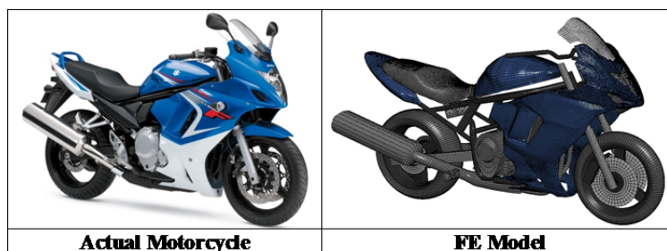
FIGURE 1 Suzuki GSX-650F motorcycle – actual motorcycle and FE model.
