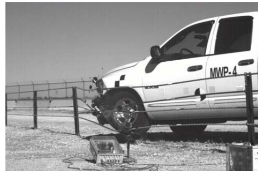
3rd cable pushed down by post
