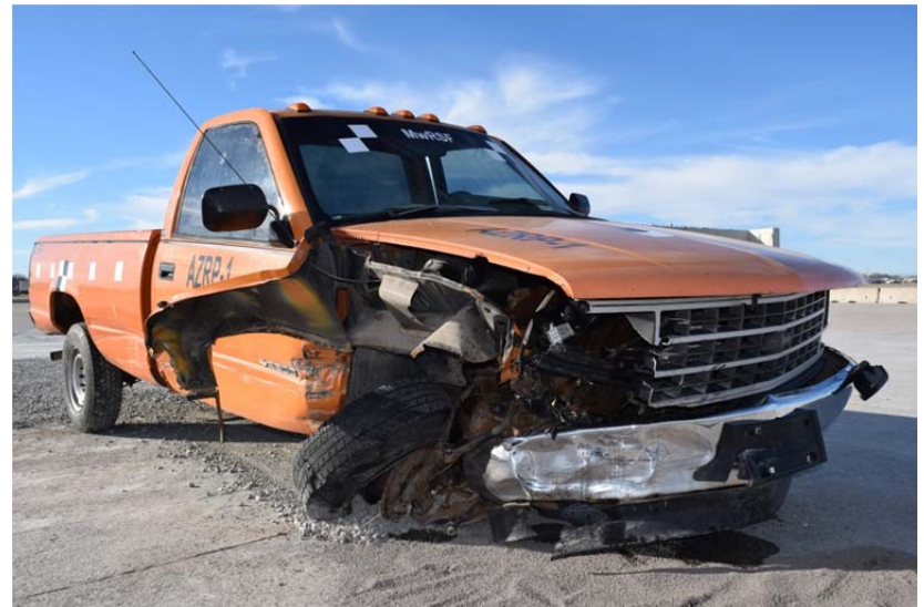
FIGURE 5 Vehicle damage and barrier damage, Test AZRP-1.
