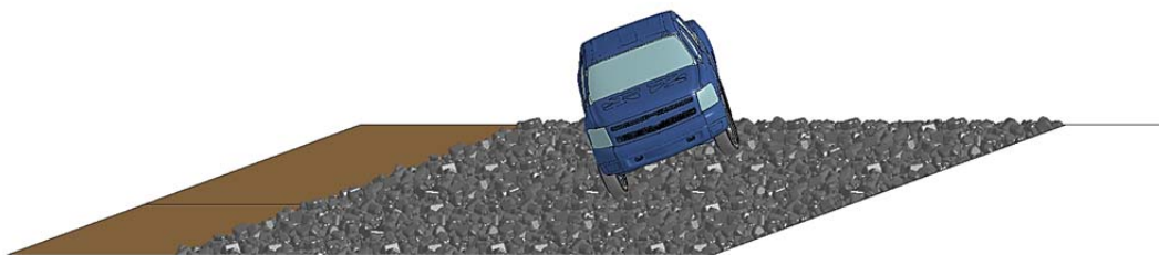
Silverado Pickup Truck Traversing on 1V:3H Slope at 45 mph
