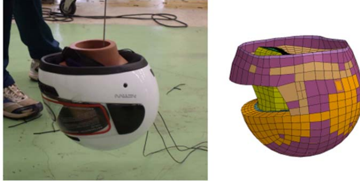
FIGURE 6 Head and helmet drop test, experimental (left) and numerical (right).
