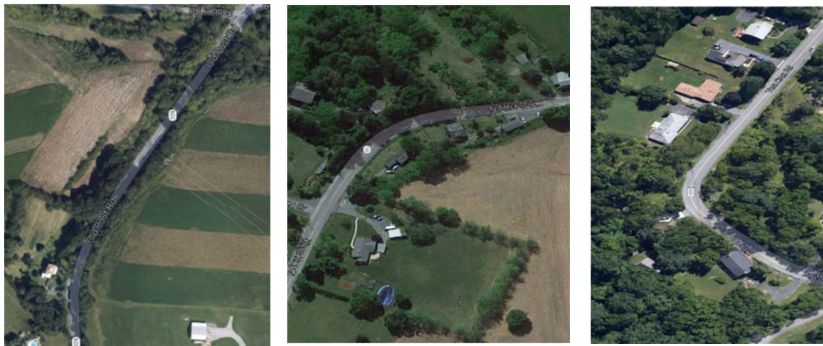
FIGURE 3 Examples of Low ( \theta = 150-180^\circ ), Medium ( \theta = 120-150^\circ ), and High ( \theta = 0-120^\circ ) Curvature Roadway Sites
