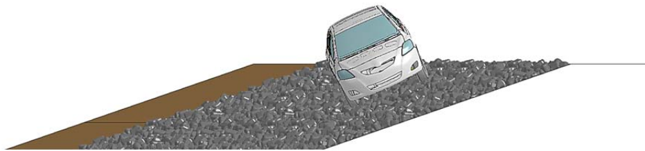
Toyota Yaris Traversing on 1V:3H Slope at 45 mph
