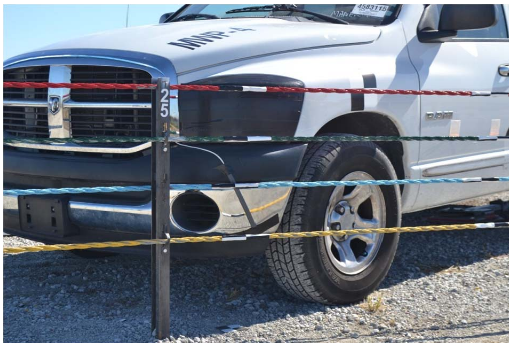
FIGURE 2 Modified Four-Cable, Median Barrier System with 38-in. Top Cable and 2270P Pickup Truck – Test No. MWP-4.
