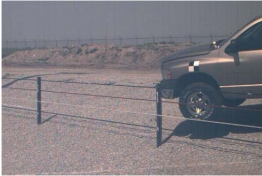
Top cable on back side of post
