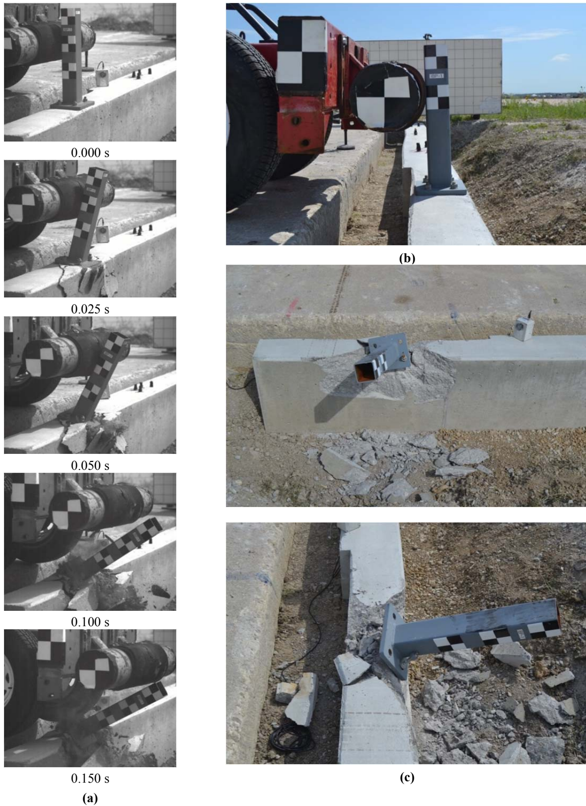
FIGURE 5 Test No. IBP-1, Original BR27C anchorage: (a) sequential events; (b) pre-test; and (c) system damage.
