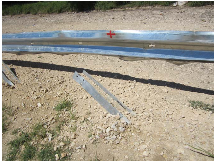
FIGURE 12 Post-Crash RFID Still Intact
