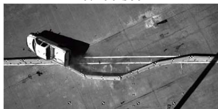
FIGURE 7 Sequential Photographs and Barrier and Vehicle Damage, Test No. NELON-2: (a) sequential events; (b) barrier damage; and (c) vehicle damage
