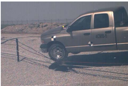
Tire overrode top cable
