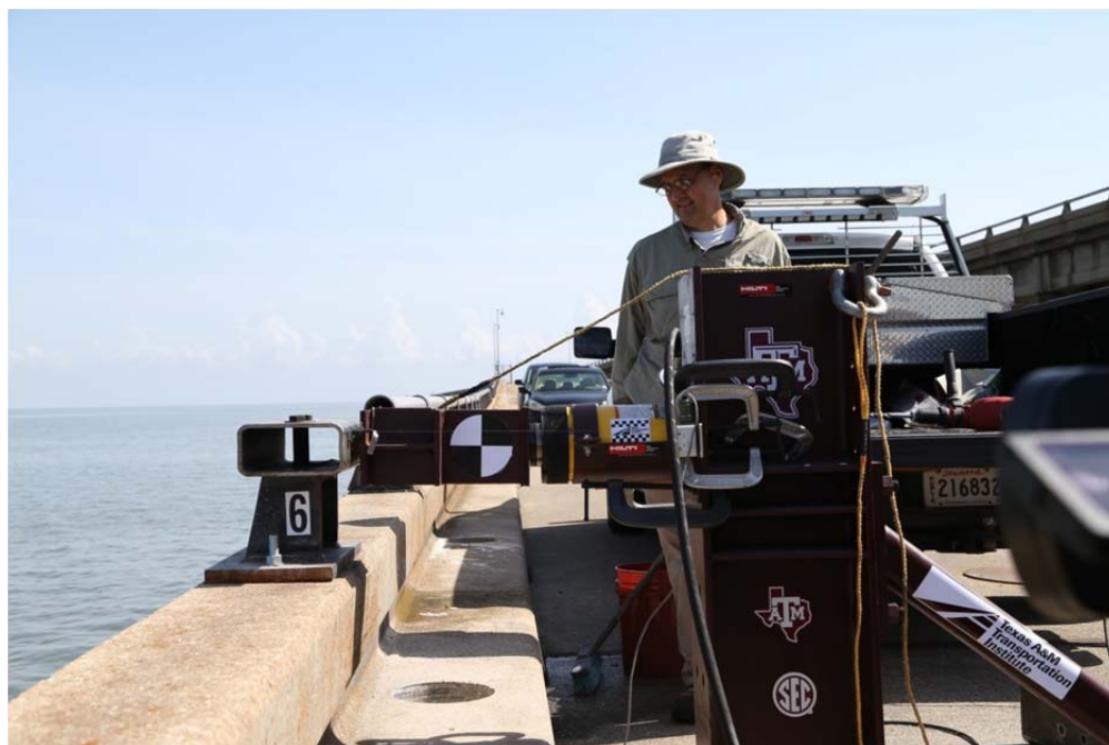
FIGURE 8 Photo of full-scale testing of steel post Retrofit Option A.
