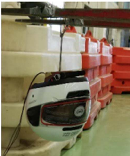
FIGURE 1 Helmet drop test configuration.
