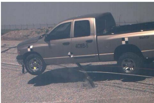
Vehicle overrode barrier
