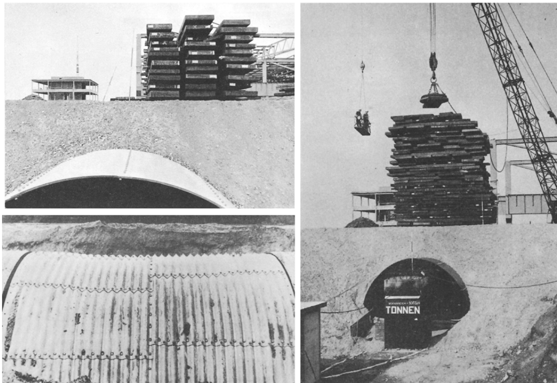
FIGURE 11 Germany 1970 pipe-arch test (6.27 x 4.03m; 4.75-mm thick plates; load = 1,079 tons).
