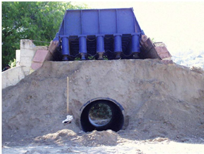
FIGURE 2 Utah State University soil cell full test, loading beams down, and load being applied to soil surface over 48-in. (1,200-mm) pipe.
