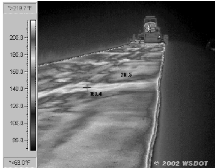
FIGURE 2 Thermal image of pavement with end-truck segregation.
