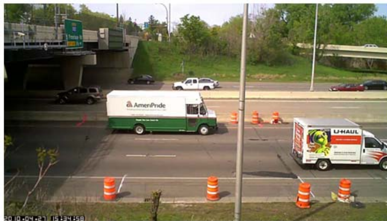
25.1 foot truck measured at 14 feet long by Canoga Microloops
