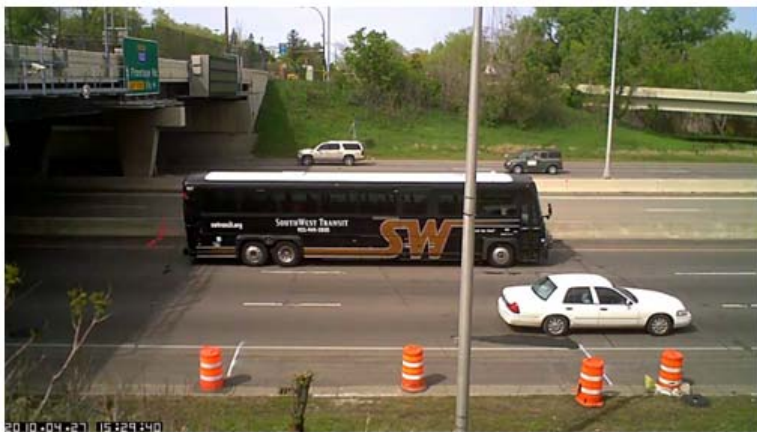
42-foot bus measured at 34 feet long by Canoga Microloops.
