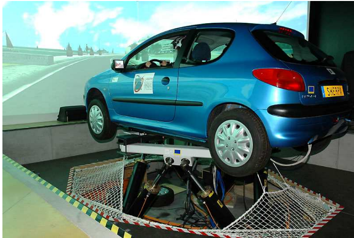
Figure 1 Driving simulator of the University of Valenciennes
