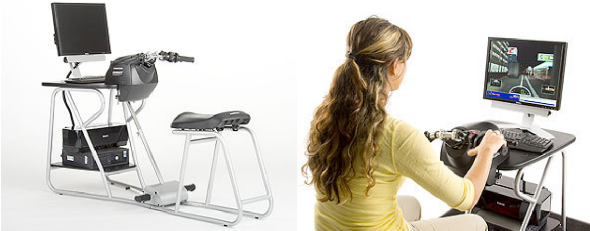
Figure 2. Honda's Riding Trainer is a computerized traffic simulator for beginning riders
