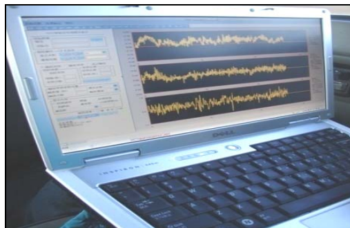
Figure 5 E-TestLab systems for analyzing the vibration acceleration signal
