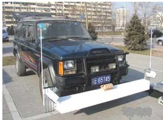
Figure 1 Multi-function laser road condition test vehicle
