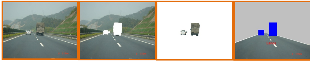
(a) Original image (b) Background image (c) Foreground (d) Focus on lanes & vehicles
